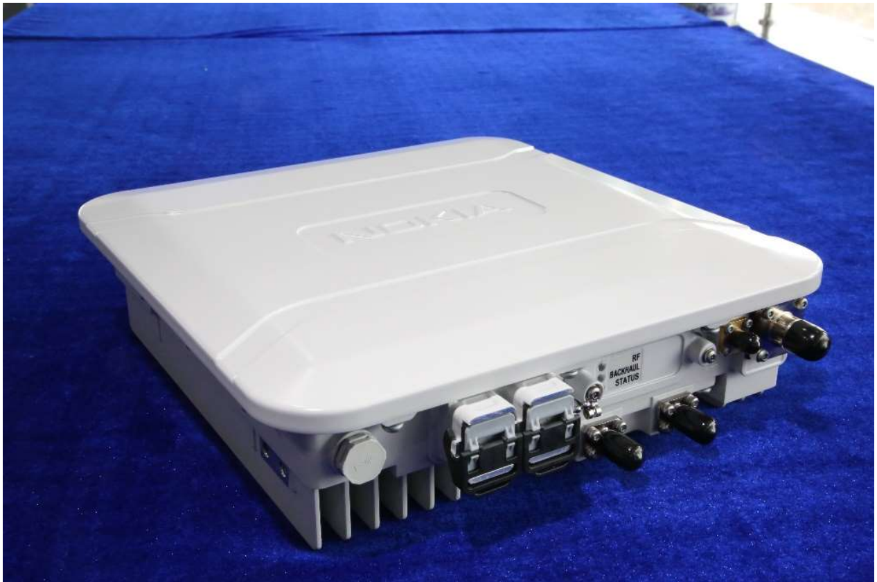
Allover photo Outline dimension : 273.5mm (L)X 269.4mm(W) X 74.3mm(H)
