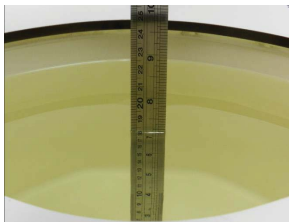
Fig 10.2 Photo of Liquid Height for Body SAR
