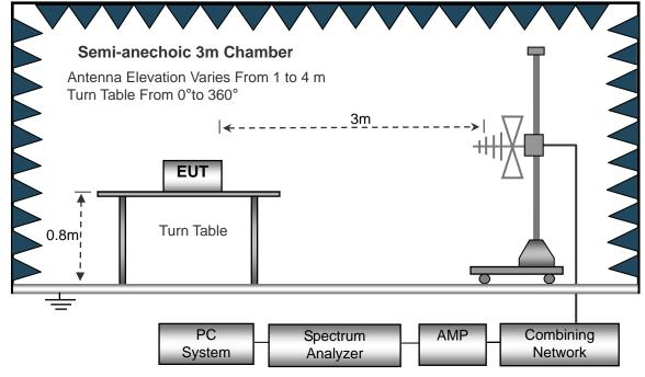
(C) Radiated Emission Test-Up Frequency Above 1GHz
