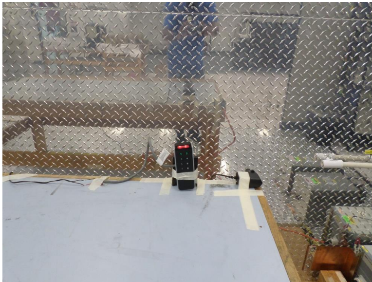
Figure 2: Conducted Emissions Limits, Pigtail, Setup EUT Front View
