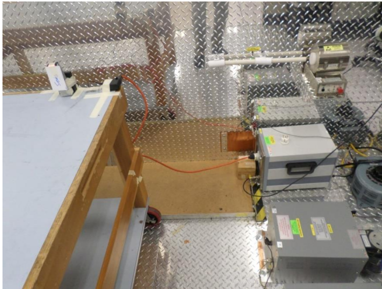
Figure 5: Conducted Emissions Limits, Terminal, Test Setup, LISN View
