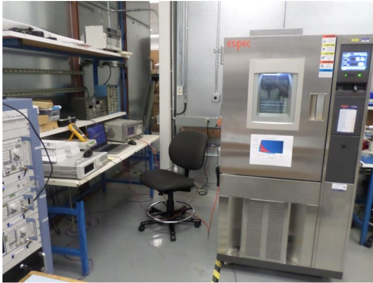
Figure 13: Frequency Stability, Terminal, Front View, Test Setup
