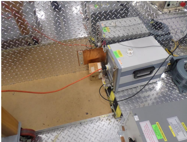
Figure 4: Conducted Emissions Limits, Pigtail, Setup LISN View
