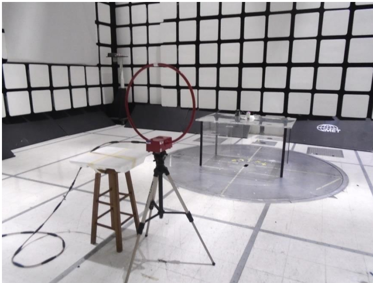
Figure 10: Radiated Spurious Emissions, 0.009 MHz – 30 MHz, Test Setup
