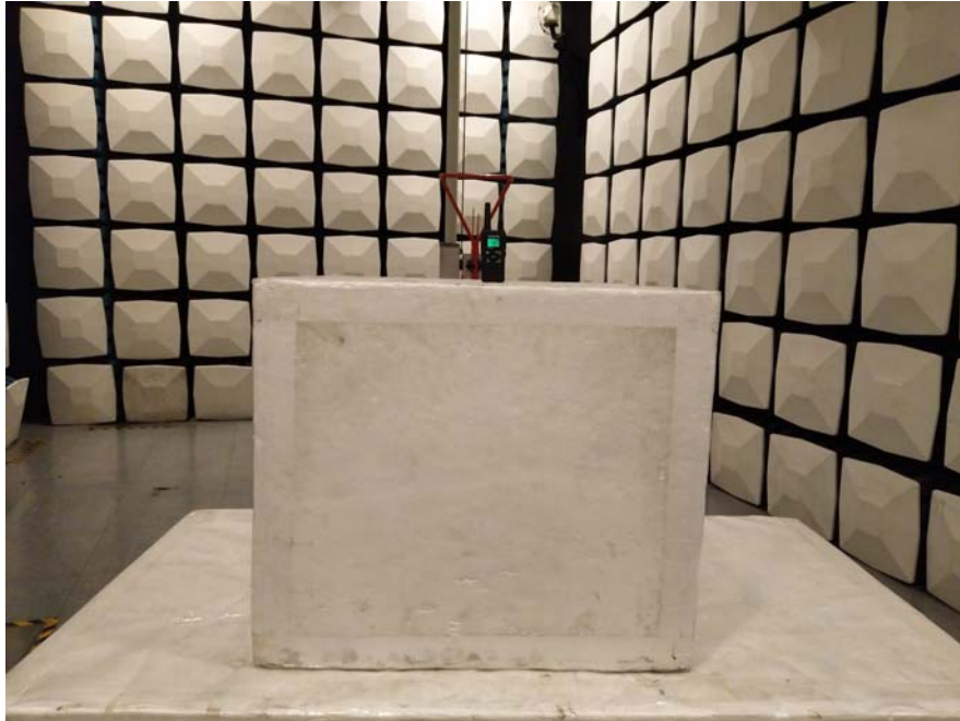
Radiated Emission Front View (Below 1 GHz)
