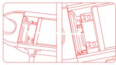
3. Remove and replace the battery. Insert the battery plug.
