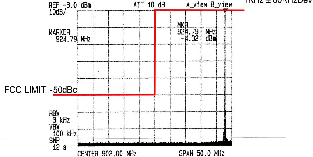
Band edge emissions: Handset CH20 EXP3241 PORT TX CH20 MAX Dev 1KHz ± 80KHzDev
