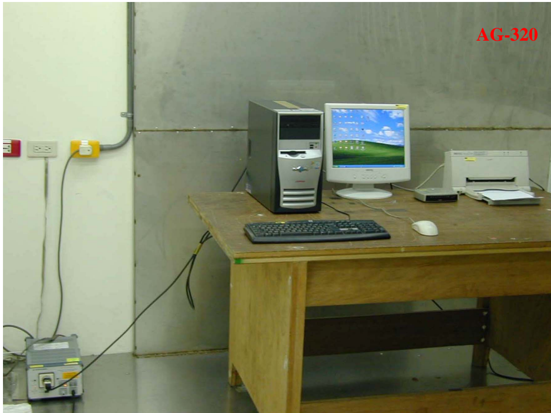
Photo 1: Conducted Emission Test Set-up photo
