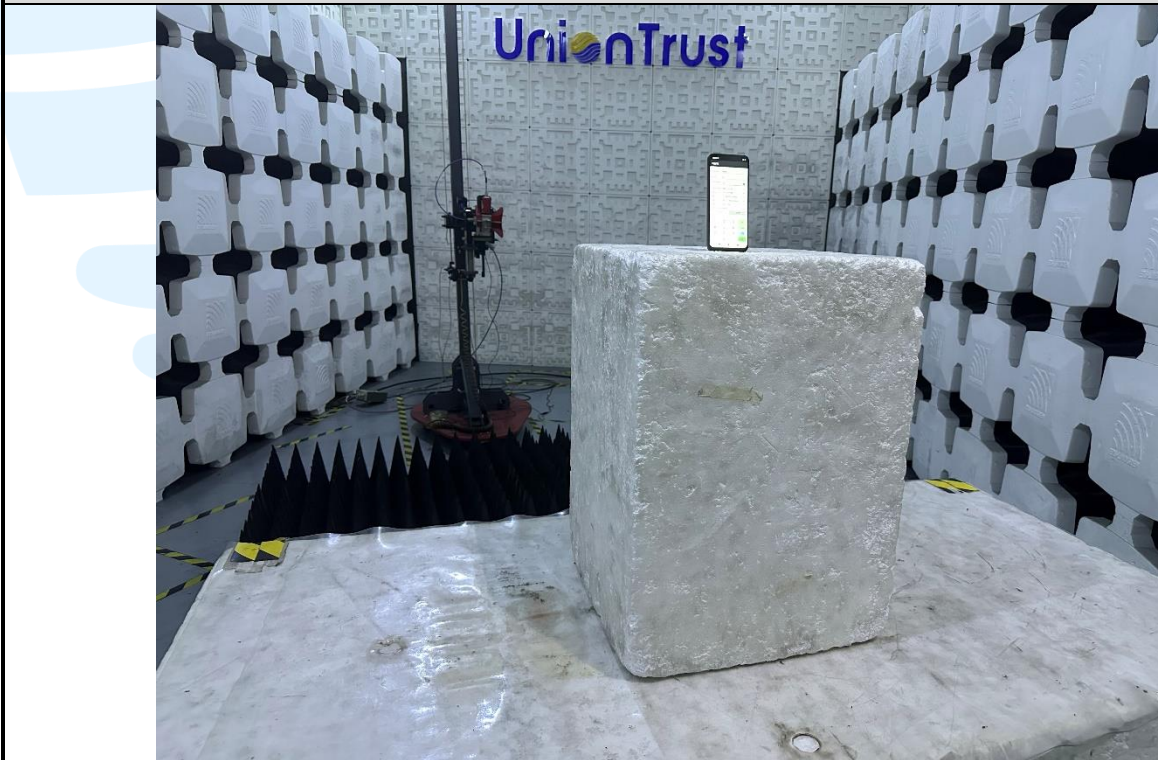
Radiated emission Test Setup (Above 1 GHz)
