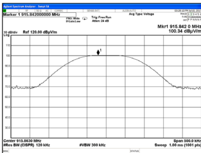
Plot 7.5.10 Field strength of carrier at mid frequency and Unom
