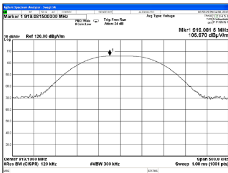
Plot 7.5.14 Field strength of carrier at high frequency and Unom
