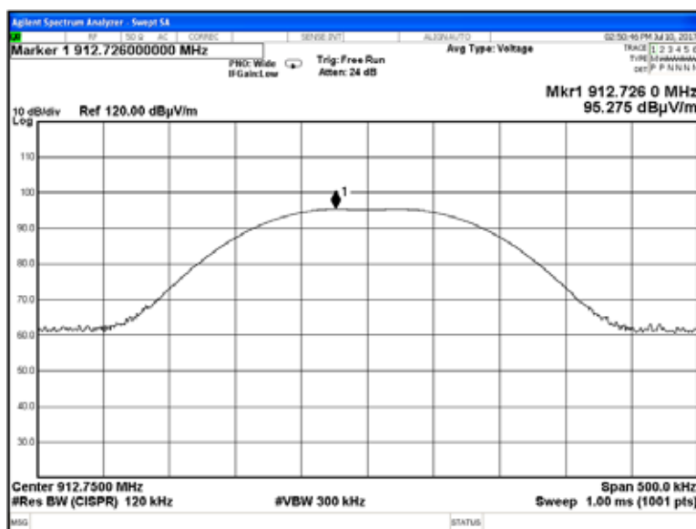
Plot 7.5.4 Field strength of carrier at low frequency and Unom
