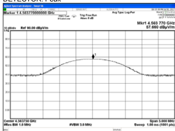
Plot 7.7.34 Radiated emission measurements at the fifth harmonic of low carrier frequency
