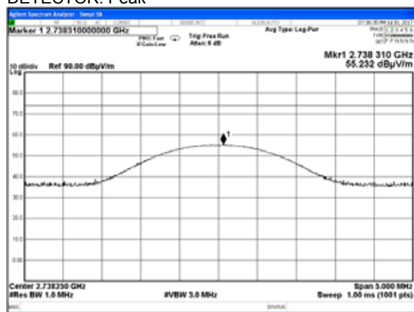
Plot 7.7.22 Radiated emission measurements at the third harmonic of low carrier frequency
