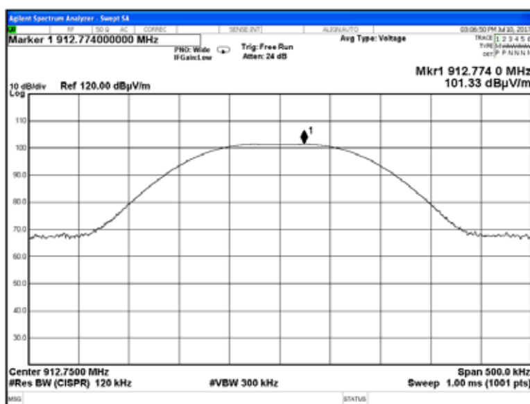
Plot 7.5.6 Field strength of carrier at low frequency and Unom
