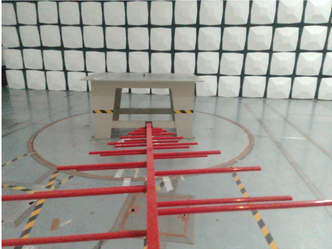
Radiated Emission Below 1GHz View
