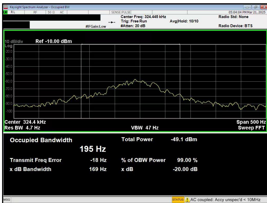
Test Plots of Occupied Bandwidth
