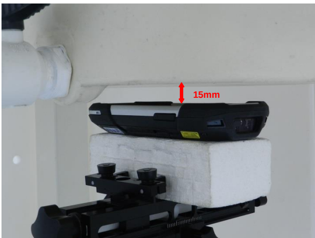
Front, Test Separation 15 mm
