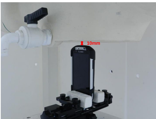
Top Side, Test Separation 10 mm
