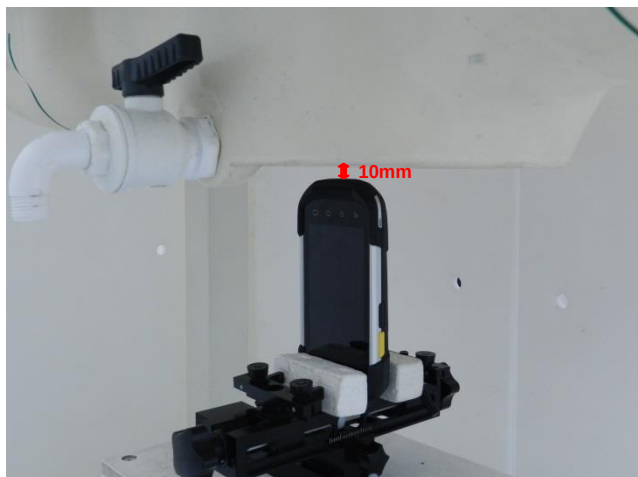
Bottom Side, Test Separation 10 mm
