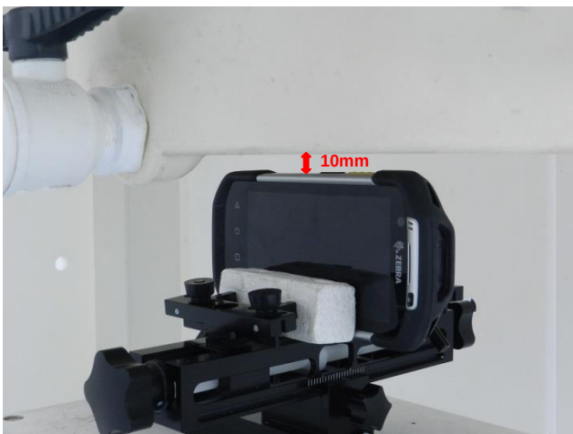
Left Side, Test Separation 10 mm
