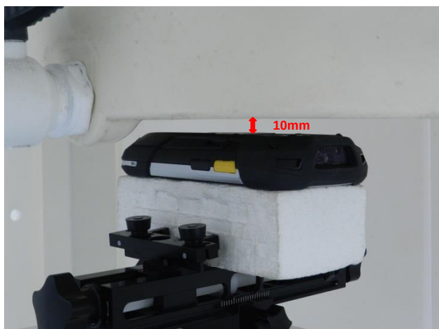
Back, Test Separation 10 mm
