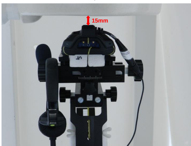
Back with Earphone 2, Test Separation 15 mm
