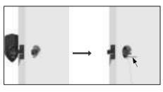
06. Insert the Exterior Assembly into the door hole. Route the cable below the latch.
