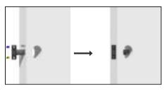
03. Put the deadbolt into the hole digged on the door. Fix it on the door with two self-tapping screws.
