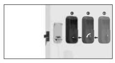
10. If the latch bolt is on the left, rotating knob to the left as shown . Otherwise, turn right
