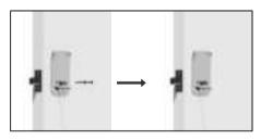
08. Fix the mounting plate on the door with two pan head screws.
