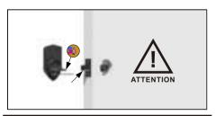
05. Turn and keep the spindle in a vertical. Please make sure the latch bolt is out before installation.
