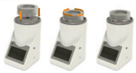
To fit the sieve head, align the flat spots at the bottom of the sieve head with the bayonet pins on the top of the iVAS Roam, then lower the sieve head onto the iVAS Roam and twist until the sieve head is held securely. To remove the sieve head, twist until it becomes loose and lift off.
