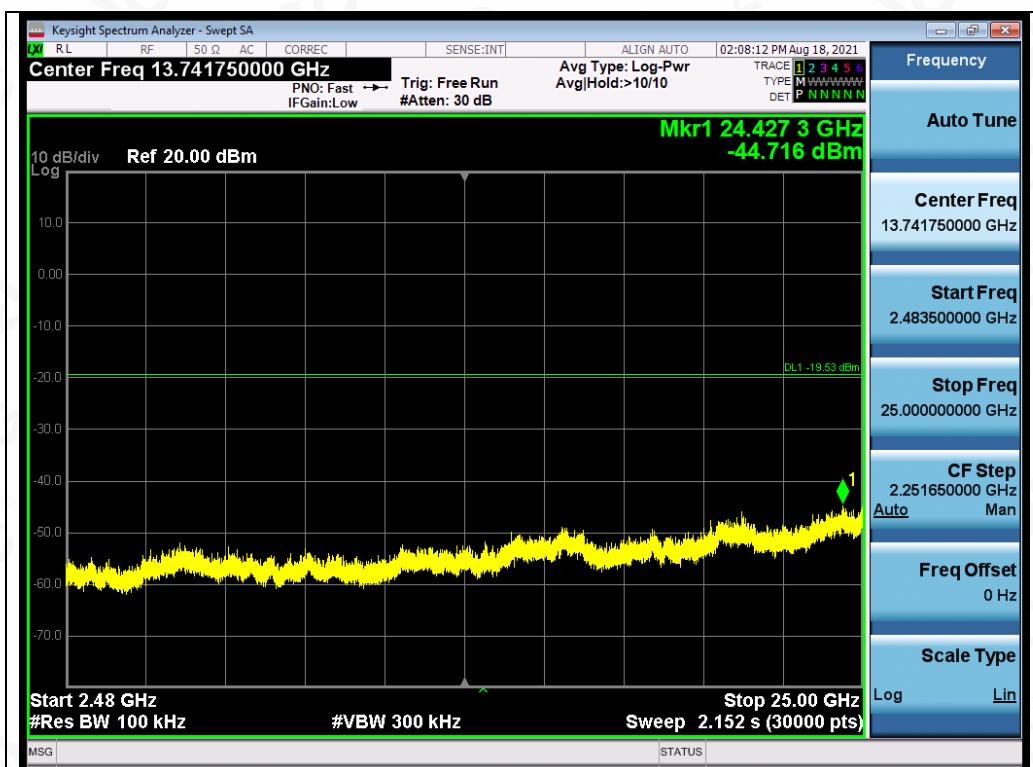
Test_Graph_EDR_ANT1_2441_2Mbps_Higher Band Emissions
