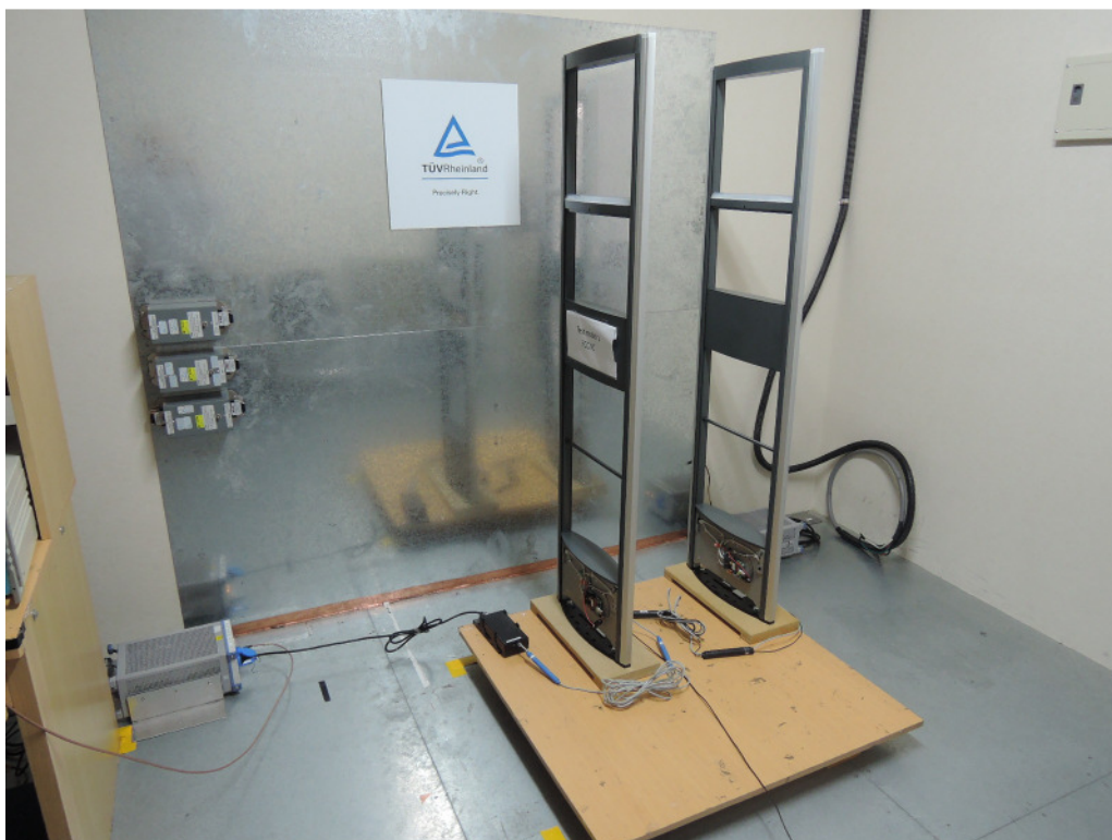
Photograph 5: Set-up for for Mains Conducted testing Front
