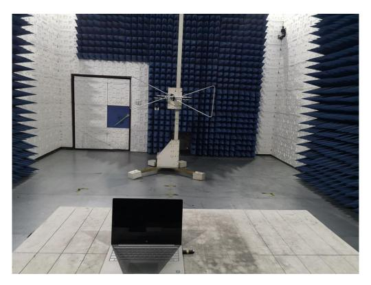
RADIATED EMISSION TEST SETUP ABOVE 1GHZ
