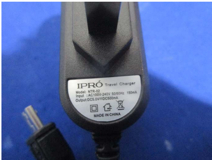
EUT – Adapter Label View
