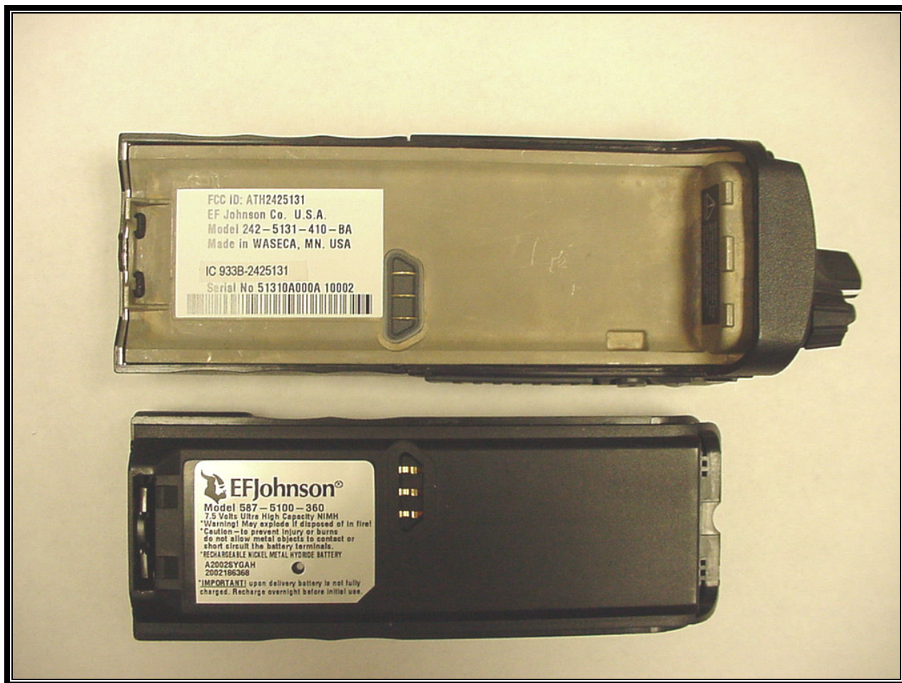
PHOTOGRAPH 1: FCC ID / IC ID LABEL SAMPLE & LOCATION
