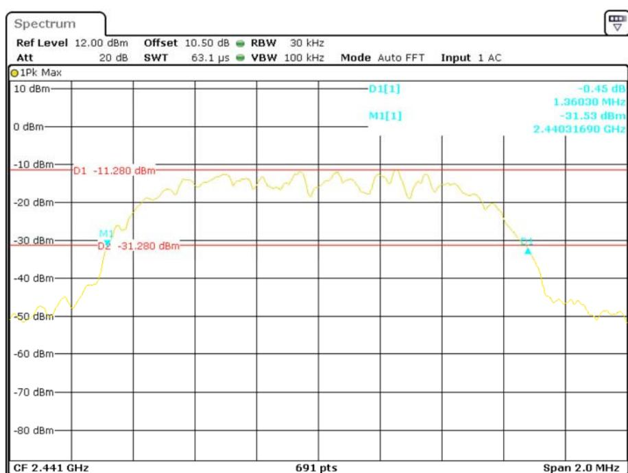
**EDR ( $\pi/4$ -DQPSK): High Channel**
