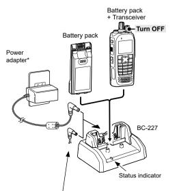
The OPC-515L\* (for a 13.8 V power source) or the CP-23L (for a 12 V cigarette lighter socket) can be used instead of the power adapter
