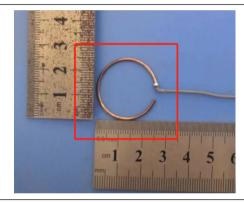
The antenna is Metal loop antenna.
