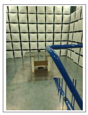
Radiated Spurious Emissions: 1 GHz to 18 GHz
