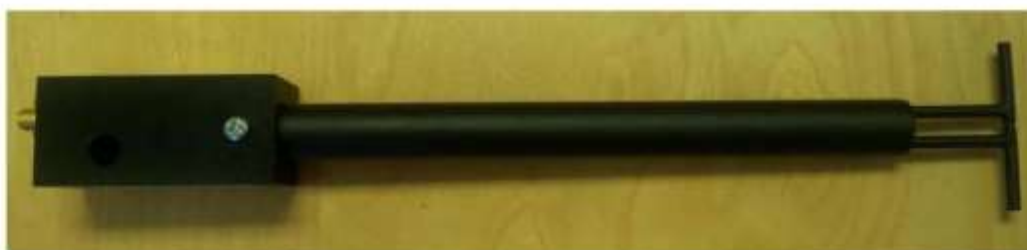
Figure 1 – MVG COMOSAR Validation Dipole
