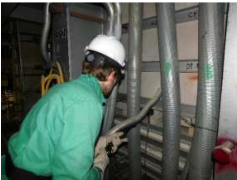
Figure 1 - FTS200 being used to measure sidewall where the FTS400 cannot fit.
