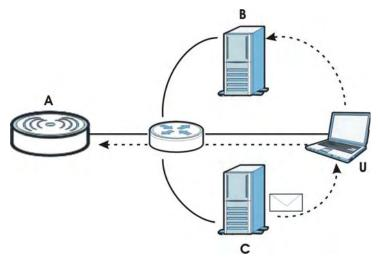
The figure above illustrates three ways to access logs. The user  $(\mathbf{U})$  can access logs directly from the NWA  $(\mathbf{A})$  via the Web configurator. Logs can also be located in an external log server  $(\mathbf{B})$ . An email server  $(\mathbf{C})$  can also send harvested logs to the user's email account.
