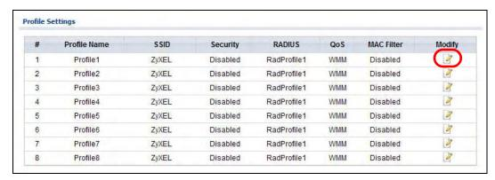
3 Rename the Profile Name and SSID as SSID01. Click Apply.
