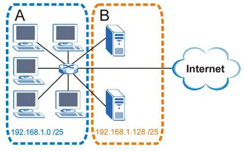
In a 25-bit subnet the host ID has 7 bits, so each sub-network has a maximum of  $2^7 - 2$  or 126 possible hosts (a host ID of all zeroes is the subnet's address itself, all ones is the subnet's broadcast address).
