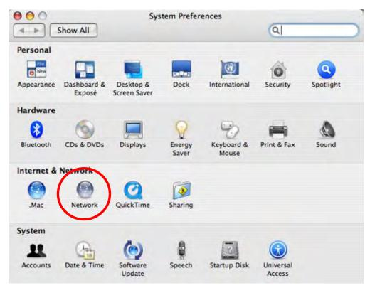
3 When the **Network** preferences pane opens, select **Built-in Ethernet** from the network connection type list, and then click **Configure**.
