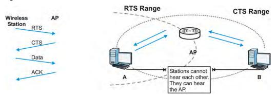
When station **A** sends data to the AP, it might not know that the station **B** is already using the channel. If these two stations send data at the same time, collisions may occur when both sets of data arrive at the AP at the same time, resulting in a loss of messages for both stations.
