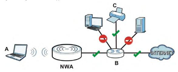
MAC addresses that are not listed in the layer-2 isolation table are blocked from communicating with the NWA's wireless clients except for broadcast packets. Layer-2 isolation does not check the traffic between wireless clients that are associated with the same AP. Intra-BSS Traffic allows wireless clients associated with the same AP to communicate with each other.
