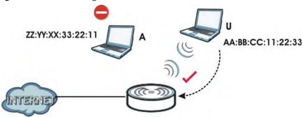
In the figure above, wireless client  $\bf U$  is able to connect to the Internet because its MAC address is in the allowed association list specified in the NWA. The MAC address of client A is either denied association or is not in the list of allowed wireless clients specified in the NWA.
