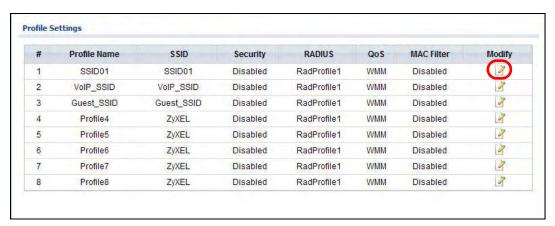
2 Select SecProfile1 as SSID01's security profile. Select the Hidden SSID checkbox as you want only authorized company employees to use this network, so there is no need to broadcast the SSID to wireless clients scanning the area.
