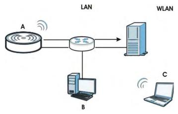
In the figure above, the NWA (A) is being managed by a desktop computer (B) connected via LAN (Land Area Network). It is also being accessed by a notebook (C) connected via WLAN (Wireless LAN).
