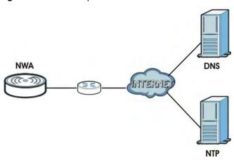
In the figure above, the NWA connects to a Domain Name Server (DNS) server to avail of a domain name. It also connects to an Network Time Protocol (NTP) server to set the time on the device.
