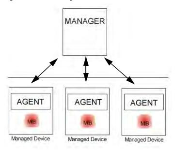
An SNMP managed network consists of two main types of component: agents and a manager.
