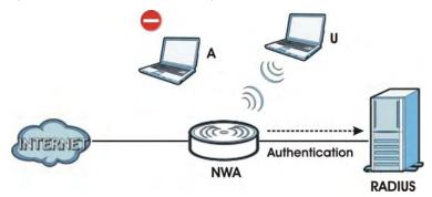
In the figure above, wireless clients  $\bf A$  and  $\bf B$  are trying to access the Internet via the NWA. The NWA in turn queries the RADIUS server if the identity of clients  $\bf A$  and  $\bf U$  are allowed access to the Internet. In this scenario, only client  $\bf U$ 's identity is verified by the RADIUS server and allowed access to the Internet.
