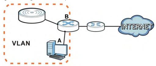
In the figure above, to access and manage the NWA from computer **A**, the NWA and switch **B**'s ports to which computer A and the NWA are connected should be in the same VLAN.
