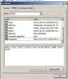
4 Use a secure method to verify that the certificate owner has the same information in the **Thumbprint Algorithm** and **Thumbprint** fields. The secure method may vary according to your situation. Possible examples would be over the telephone or through an HTTPS connection.
