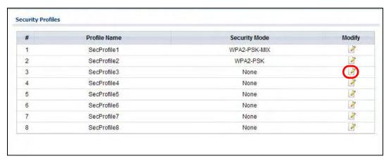
6 Select **WPA-PSK** in the **Security Mode** field. WPA-PSK provides strong security that is supported by most wireless clients. Even though your **Guest\_SSID** clients do not have access to sensitive information on the network, you should not leave the network without security. An attacker could still cause damage to the network or intercept unsecured communications or use your Internet access for illegal activities.
