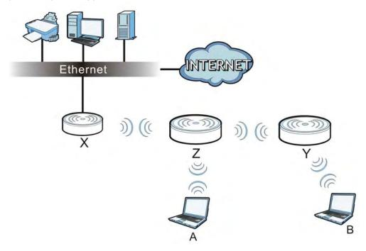
When the NWA is in Repeater mode, universal repeater security between the NWA and other repeater is independent of the security between the wireless clients and the AP or repeater. If you do not enable universal repeater security, traffic between APs is not encrypted. When universal repeater security is enabled, both APs and repeaters must use the same pre-shared key. See Section 6.6 on page 76 for more details.
