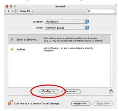
4 For dynamically assigned settings, select **Using DHCP** from the **Configure IPv4** list in the **TCP/IP** tab.
