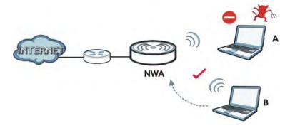
In the figure above, the NWA checks the identity of devices before giving them access to the network. In this scenario, Computer  $\bf A$  is denied access to the network, while Computer  $\bf B$  is granted connectivity.
