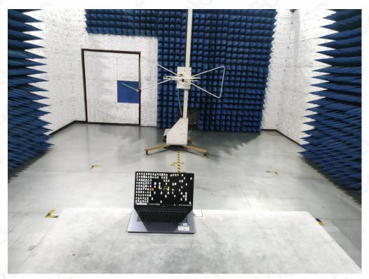
RADIATED EMISSION TEST SETUP ABOVE 1GHz
