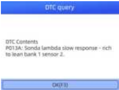
Figure 5-38 Sample Trouble Codes Screen
