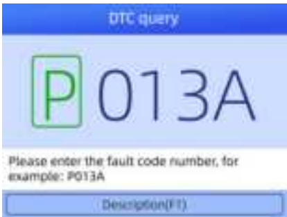
Figure 5-37 Sample DTC Lookup Screen
