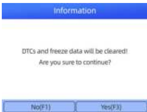
Figure 5-5 Sample Erase Codes Screen
