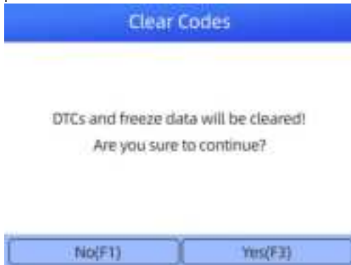
Figure 4-20 Sample Clear Codes Screen
