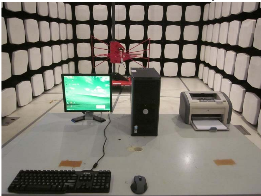
Measurement of Radiated Emission Test Set Up
