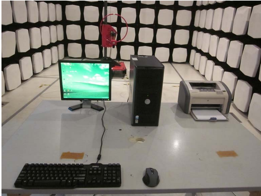
Measurement of Radiated Emission Test Set Up
