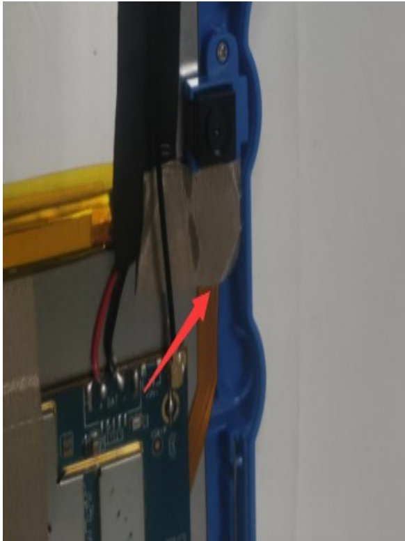
Camera cable is shielded by conductive cloth
