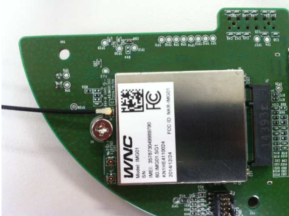
Connect to LTE primary antenna
