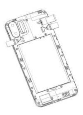
2) Remove the battery, and install SIM and SD cards, place the cards with chip facing downwards, and then slide it into its slot. Make sure that it is correctly inserted.
