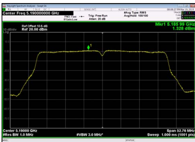
U-NII-1 Power spectral density-802.11 ac(40MHz),5190MHz,Ant0
