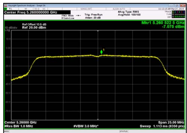
U-NII-2a Power spectral density-802.11 1n(20MHz),5260MHz,Ant1
