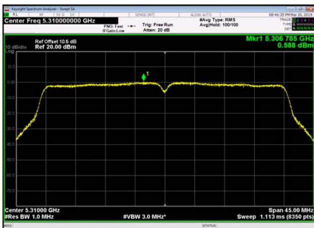
U-NII-2a Power spectral density-802.1 1ac(40MHz),5310MHz,Ant0
