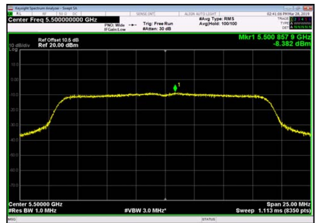
U-NII-2c Power spectral density-802.1 1ac(20MHz),5600MHz,Ant1
