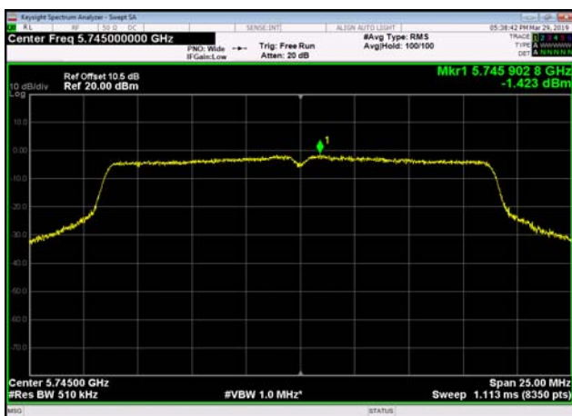
U-NII-3 Power spectral density-802.11 ac(20MHz),5745MHz,Ant0
