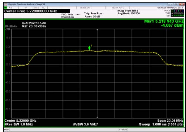
U-NII-1 Power spectral density-802.11 a(20MHz),5240MHz,Ant1
