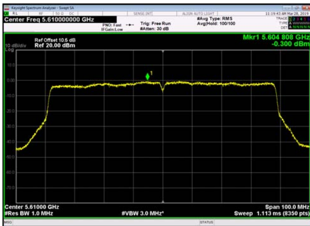
U-NII-2c Power spectral density-802.1 1ac(80MHz),5610MHz,Ant0
