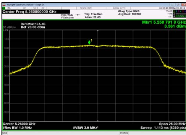
U-NII-2a Power spectral density-802.1 1a(20MHz),5300MHz,Ant0
