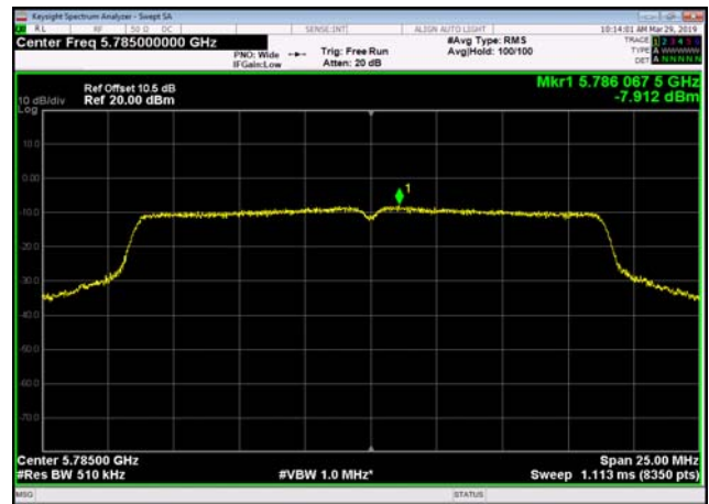
U-NII-3 Power spectral density-802.11 ac(20MHz),5825MHz,Ant1
