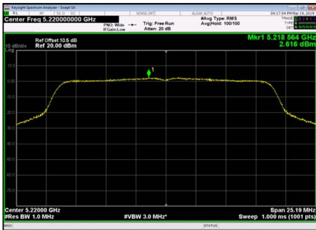
U-NII-1 Power spectral density-802.11 a(20MHz),5240MHz,Ant0
