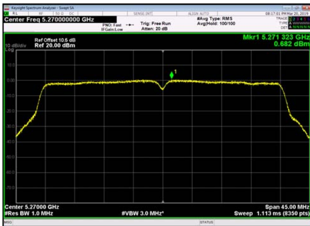
U-NII-2a Power spectral density-802.1 1n(40MHz),5270MHz,Ant0
