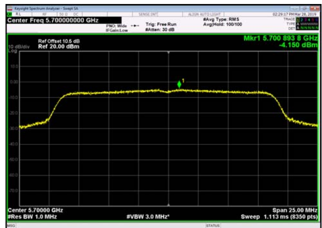
U-NII-2c Power spectral density-802.1 1n(40MHz),5510MHz,Ant1
