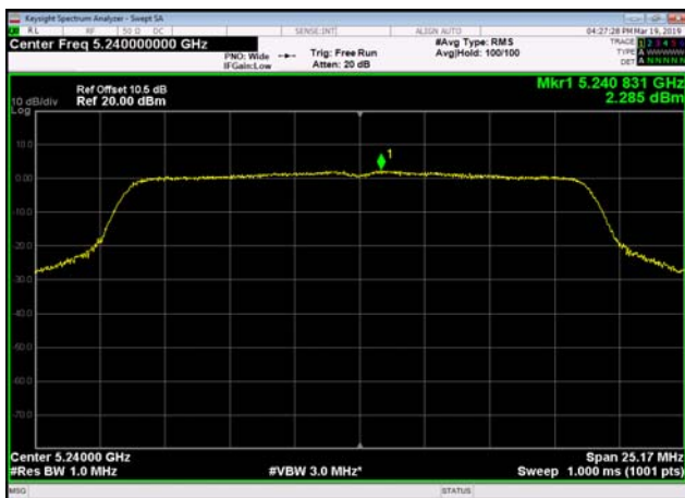
U-NII-1 Power spectral density-802.11 ac(20MHz),5180MHz,Ant0
