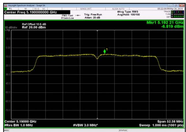
U-NII-1 Power spectral density-802.11 ac(40MHz),5190MHz,Ant1
