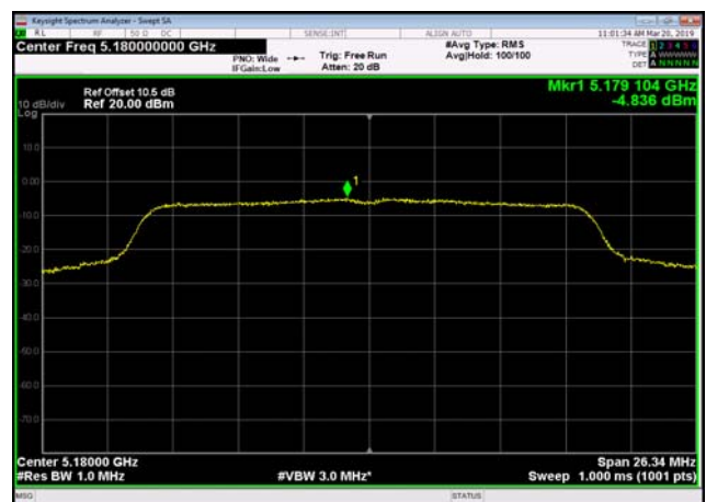
U-NII-1 Power spectral density-802.11 ac(20MHz),5180MHz,Ant1
