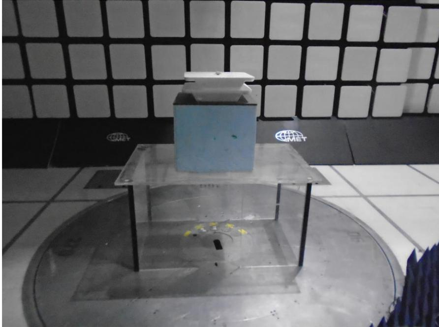
**Photograph 9. Radiated Emissions, 18 - 25 GHz, Setup Front**
