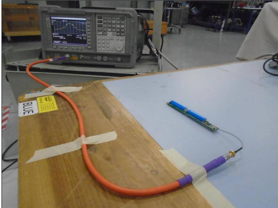
**Photograph 1. Occupied Bandwidth Setup**
