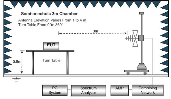
(C) Radiated Emission Test-Up Frequency Above 1GHz
