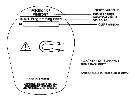
Figure 10: 47 CFR 15.19 Labelling Requirements
