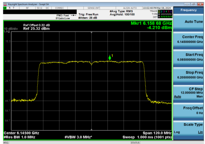
Plot 7-376. SP Power Spectral Density Plot CDD Diversity Antenna WF7b (80MHz 802.11ax RU996 (UNII Band 5) – Ch. 39)
