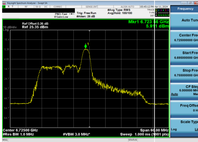
Plot 7-396. SP Power Spectral Density Plot CDD Diversity Antenna WF7b (40MHz 802.11ax RU26 (UNII Band 7) – Ch. 155)
