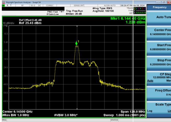
Plot 7-371. SP Power Spectral Density Plot CDD Diversity Antenna WF2a (80MHz 802.11ax RU26 (UNII Band 5) – Ch. 39)
