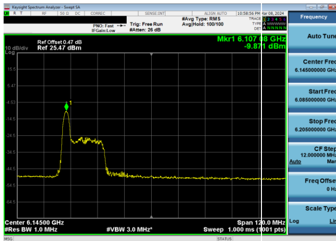
Plot 7-425. LPI Power Spectral Density Plot Antenna WF7a (80MHz 802.11ax RU26 (UNII Band 5) – Ch. 39)
