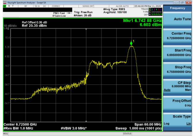
Plot 7-398. SP Power Spectral Density Plot CDD Diversity Antenna WF7b (40MHz 802.11ax RU26 (UNII Band 7) – Ch. 155)
