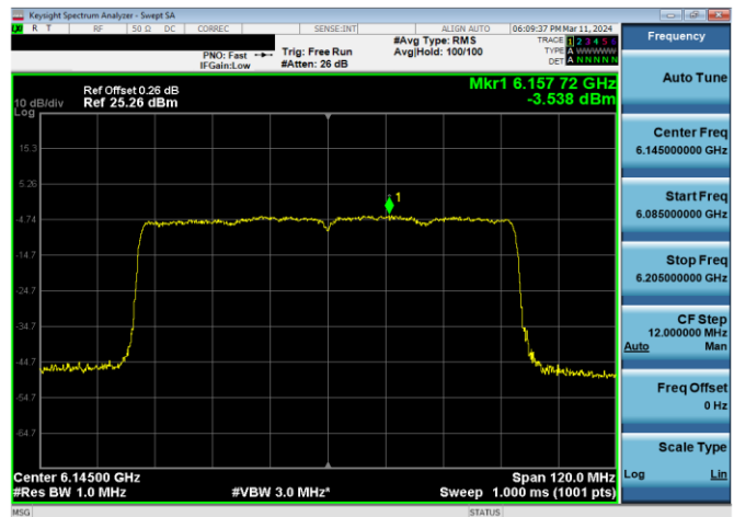
Plot 7-428. LPI Power Spectral Density Plot Antenna WF7a (80MHz 802.11ax RU996 (UNII Band 5) – Ch. 39)
