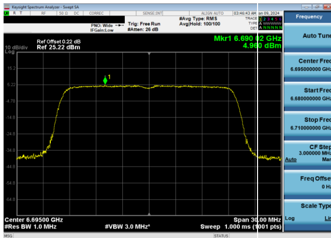
Plot 7-391. SP Power Spectral Density Plot CDD Diversity Antenna WF2a (20MHz 802.11ax RU242 (UNII Band 7) – Ch. 149)
