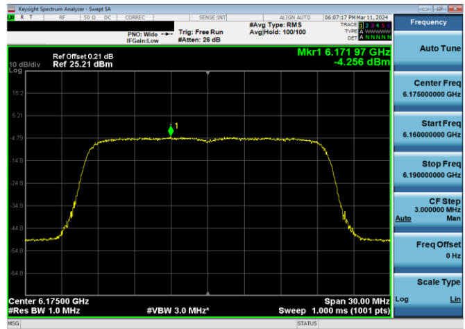
Plot 7-420. LPI Power Spectral Density Plot Antenna WF7a (20MHz 802.11ax RU242 (UNII Band 5) – Ch. 45)
