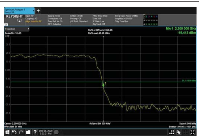
Figure 160: 16QAM 5MHz B.W.; 2197.5MHz Upper Edge – 4G
