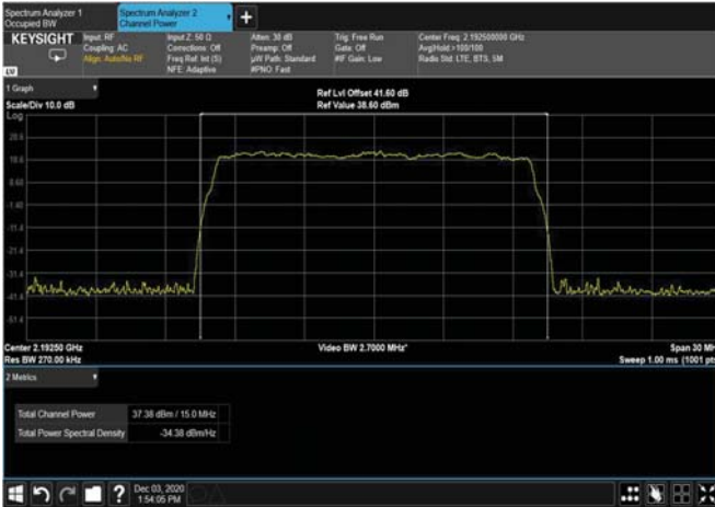
Figure 92: 16QAM 15MHz B.W; 2192.5MHz – 4G
