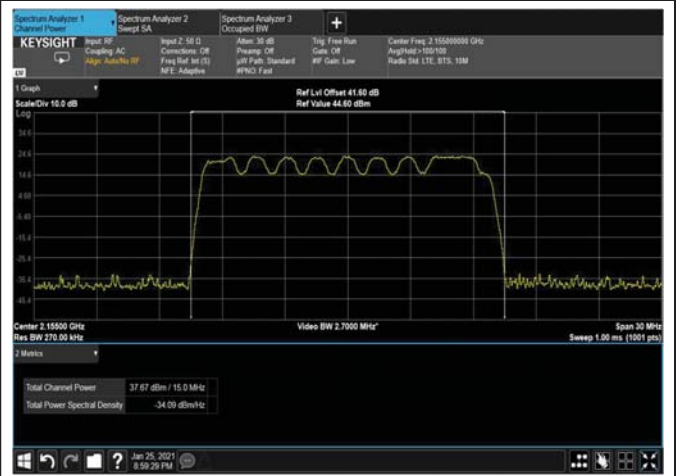
Figure 78: QPSK 15MHz B.W; 2155.0MHz, 30kHz
