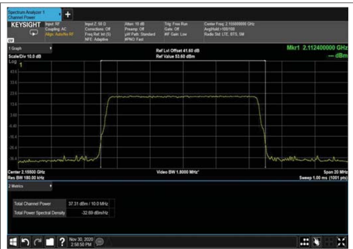
Figure 97: 64QAM 10MHz; 2155MHz – 4G
