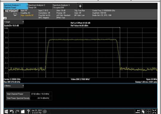
Figure 60: 256QAM 15MHz B.W; 2192.5MHz, 30kHz
