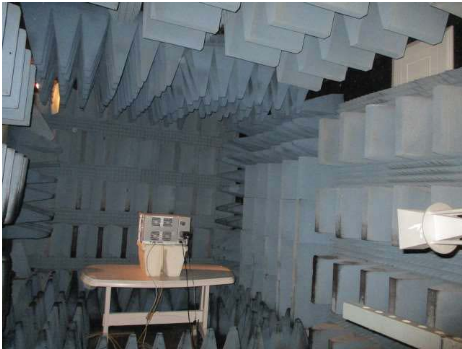
Figure 8. Radiated Emission Test 18.0-22.0GHz
