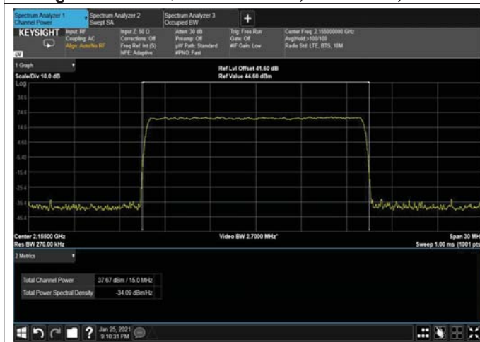
Figure 59: 256QAM 15MHz B.W; 2155.0MHz, 15kHz
