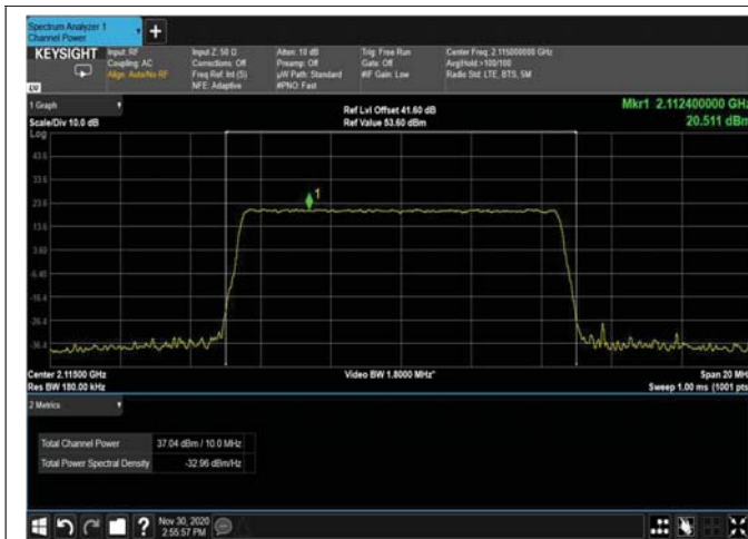
Figure 96: 64QAM 10MHz B.W; 2115MHz – 4G
