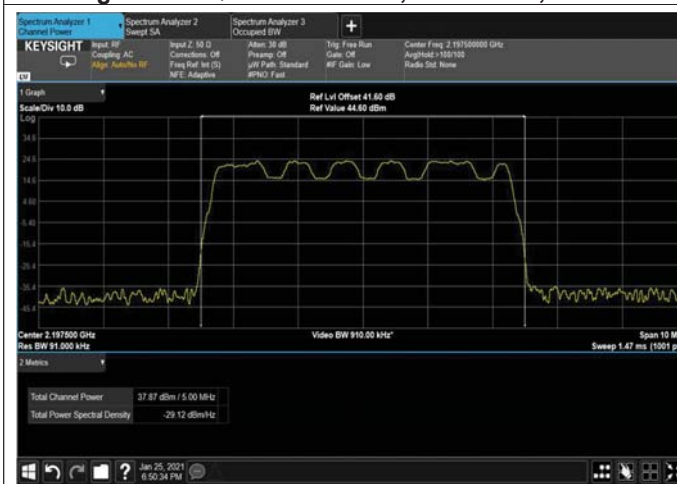
Figure 67: QPSK 5MHz B.W; 2197.5MHz, 15kHz
