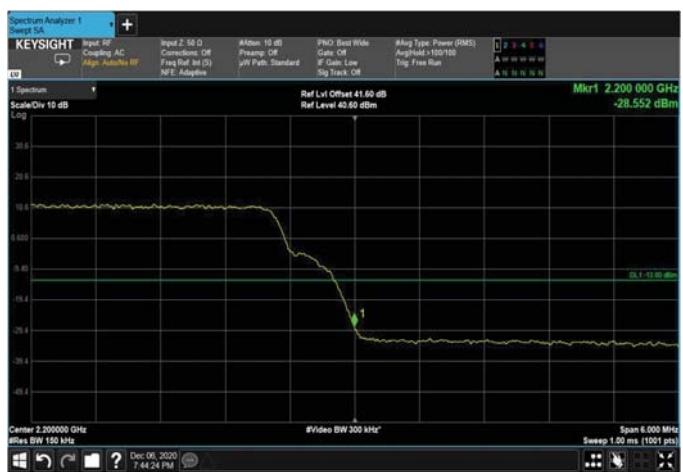
Figure 176: QPSK 15MHz B.W.; 2192.5MHz Upper Edge – 4G
