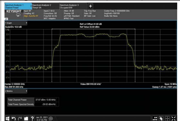
Figure 12: 16QAM 5MHz B.W; 2155.0MHz, 30kHz
