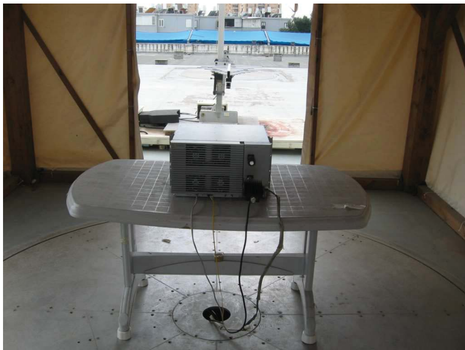
Figure 6. Radiated Emission Test 200 - 1000MHz
