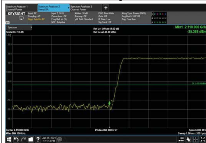
Figure 133: 64QAM 15MHz B.W.; 2117.5MHz, 30kHz Lower Edge
