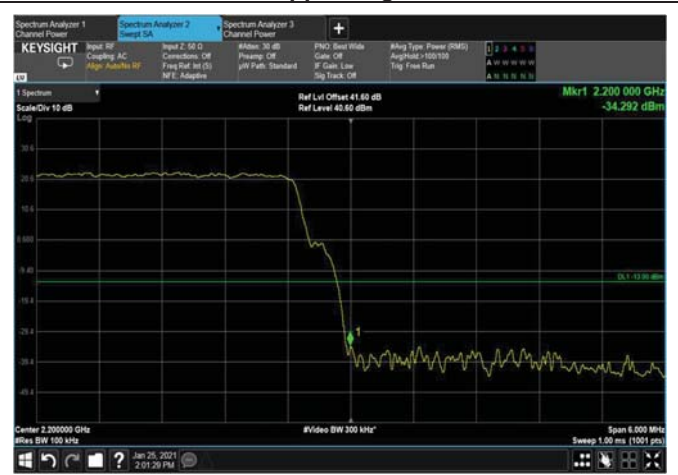
Figure 126: 64QAM 5MHz B.W.; 2197.5MHz, 30kHz Upper Edge
