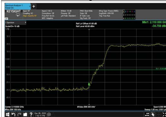
Figure 163: 16QAM 15MHz B.W.; 2117.5MHz Lower Edge – 4G
