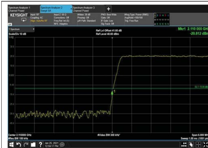
Figure 135: 256QAM 5MHz B.W.; 2112.5MHz, 15kHz Lower Edge
