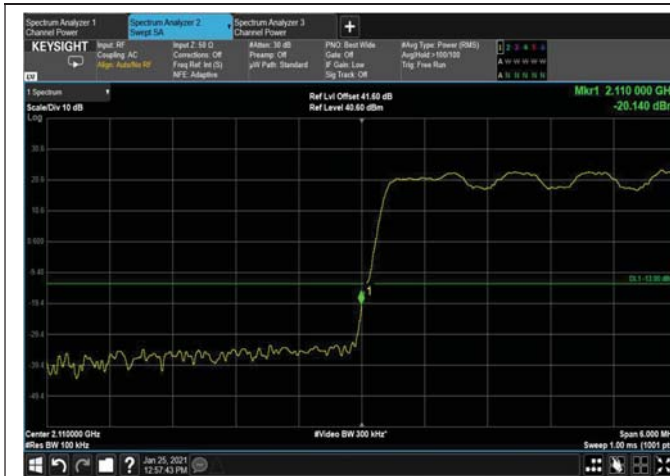
Figure 111: 16QAM 5MHz B.W.; 2112.5MHz, 15kHz Lower Edge
