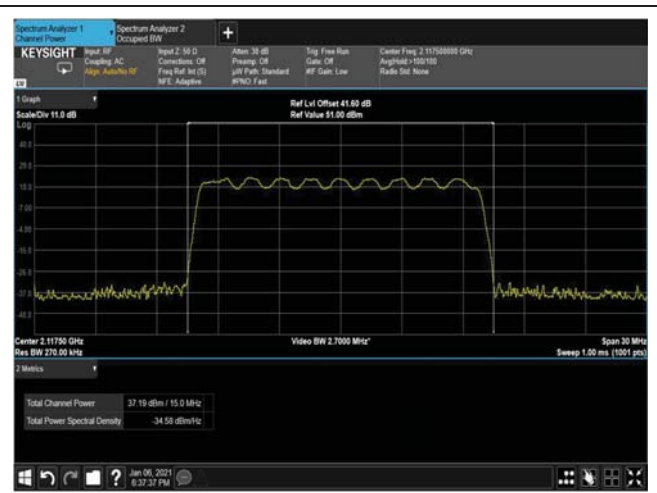
Figure 22: 16QAM 15MHz B.W; 2117.5MHz, 30kHz
