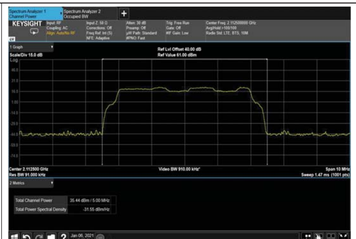
Figure 10: 16QAM 5MHz B.W; 2112.5MHz, 30kHz
