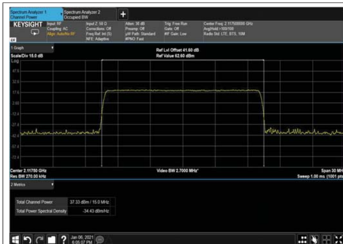
Figure 57: 256QAM 15MHz B.W; 2117.5MHz, 15kHz
