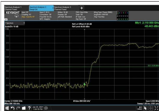
Figure 117: 16QAM 10MHz B.W.; 2115MHz, 30kHz Lower Edge
