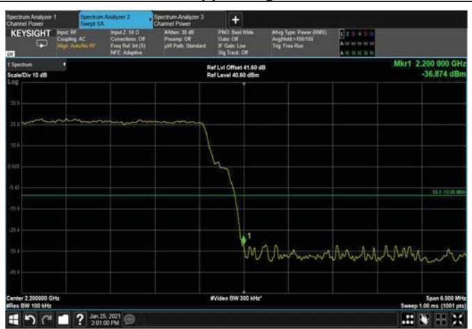
Figure 138: 256QAM 5MHz B.W.; 2197.5MHz, 30kHz Upper Edge
