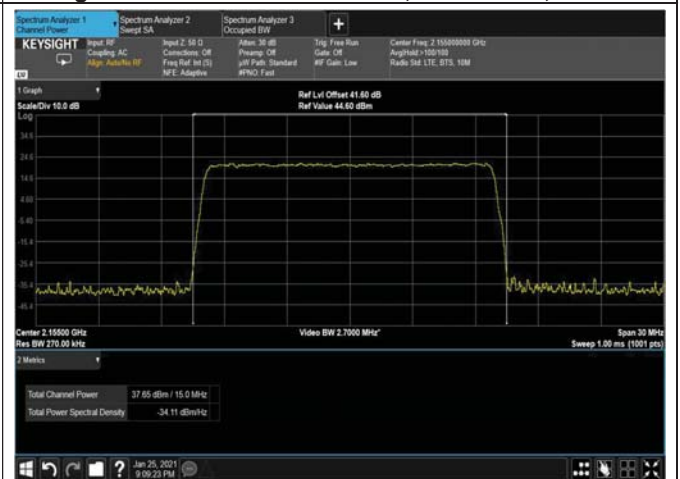
Figure 42: 64QAM 15MHz B.W; 2155.0MHz, 30kHz
