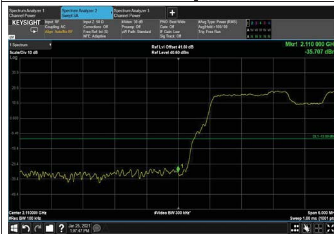
Figure 157: QPSK 15MHz B.W.; 2117.5MHz, 30kHz Lower Edge
