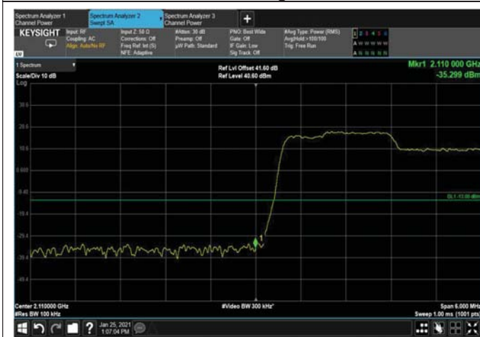
Figure 155: QPSK 15MHz B.W.; 2117.5MHz, 15kHz Lower Edge
