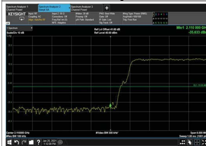
Figure 145: 256QAM 15MHz B.W.; 2117.5MHz, 30kHz Lower Edge
