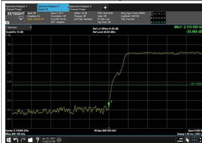
Figure 137: 256QAM 5MHz B.W.; 2112.5MHz, 30kHz Lower Edge
