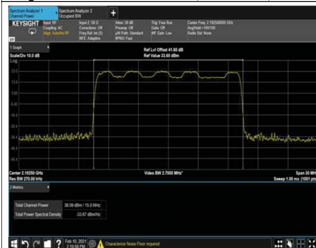
Figure 25: 16QAM 15MHz B.W; 2192.5MHz, 15 kHz
