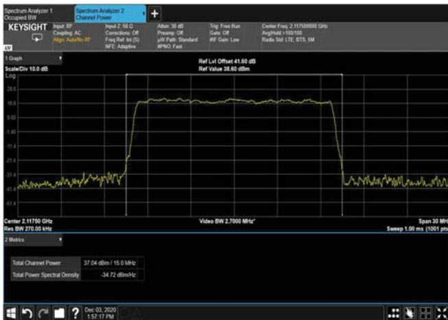
Figure 90: 16QAM 15MHz B.W; 2117.5MHz – 4G
