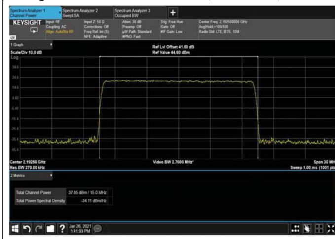
Figure 61: 256QAM 15MHz B.W; 2192.5MHz, 15kHz
