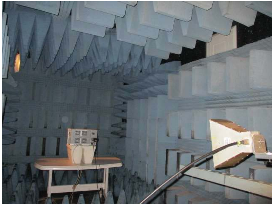
Figure 7. Radiated Emission Test 1.0 - 18.0GHz
