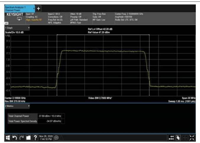
Figure 109: QPSK 15MHz B.W; 2155MHz – 4G
