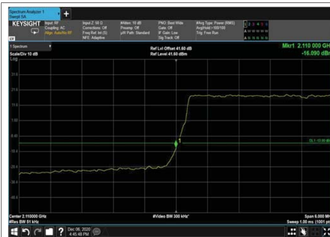
Figure 165: 64QAM 5MHz B.W.; 2112.5MHz Lower Edge – 4G
