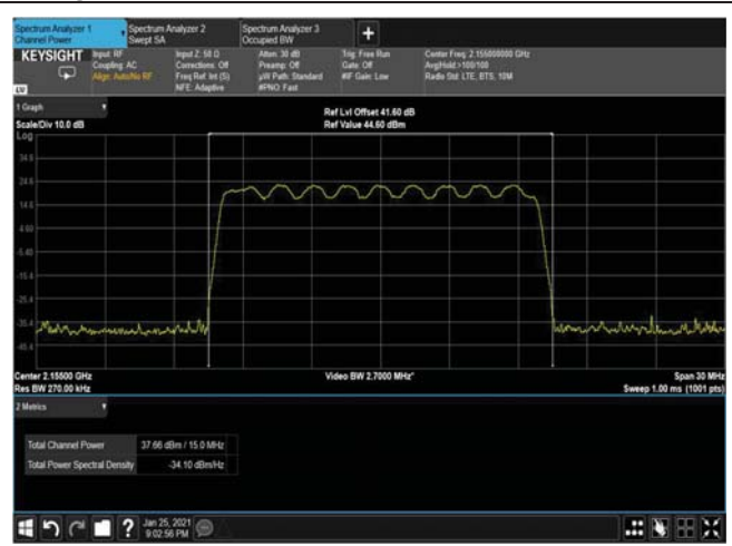
Figure 24: 16QAM 15MHz B.W; 2155.0MHz, 30kHz
