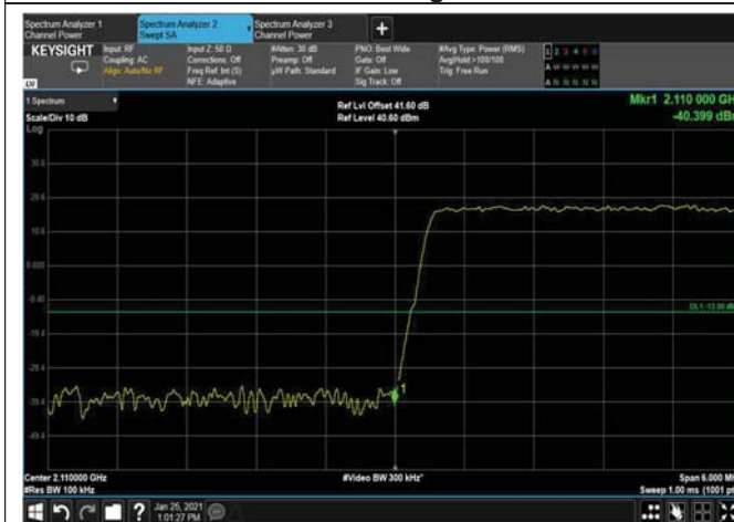
Figure 139: 256QAM 10MHz B.W.; 2115MHz, 15kHz Lower Edge
