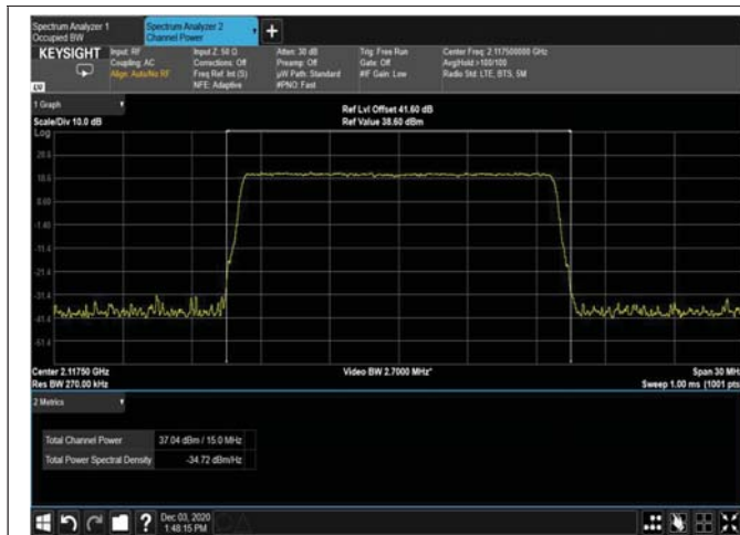
Figure 108: QPSK 15MHz B.W; 2117.5MHz – 4G
