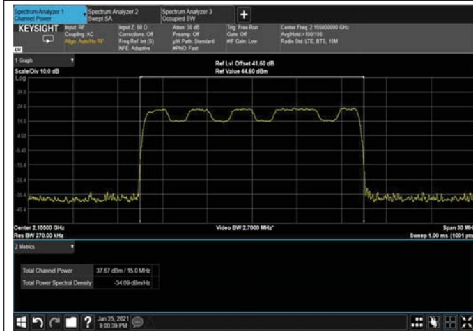
Figure 77: QPSK 15MHz B.W; 2155.0MHz, 15kHz
