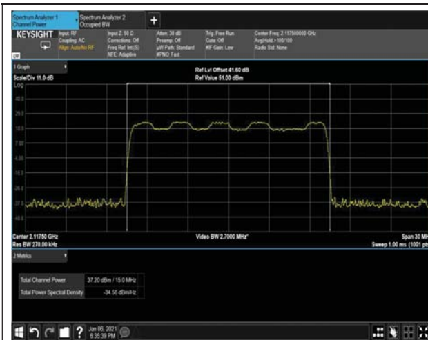
Figure 21: 16QAM 15MHz B.W; 2117.5MHz, 15kHz
