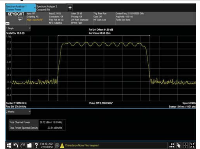
Figure 26: 16QAM 15MHz B.W; 2192.5MHz, 30kHz
