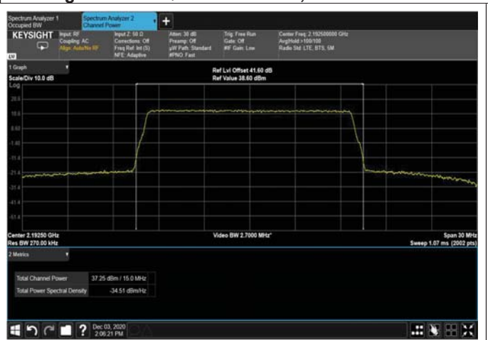
Figure 101: 64QAM 64MHz B.W; 2192.5MHz – 4G
