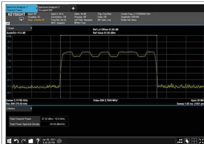
Figure 75: QPSK 15MHz B.W; 2117.5MHz, 15kHz
