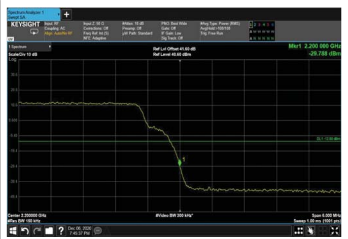
Figure 170: 64QAM 15MHz B.W.; 2192.5MHz Upper Edge – 4G
