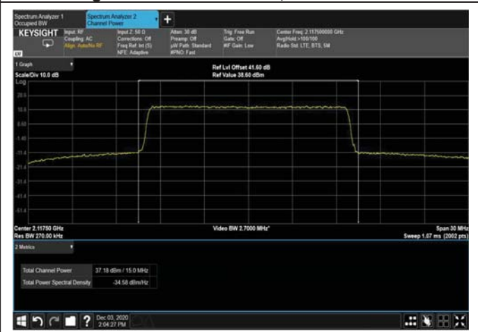
Figure 99: 64QAM 15MHz B.W; 2117.5MHz – 4G
