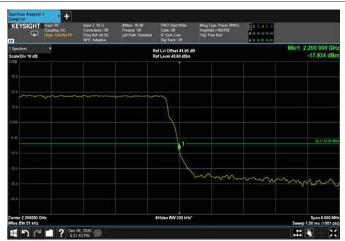
Figure 172: QPSK 5MHz B.W.; 2197.5MHz Upper Edge – 4G
