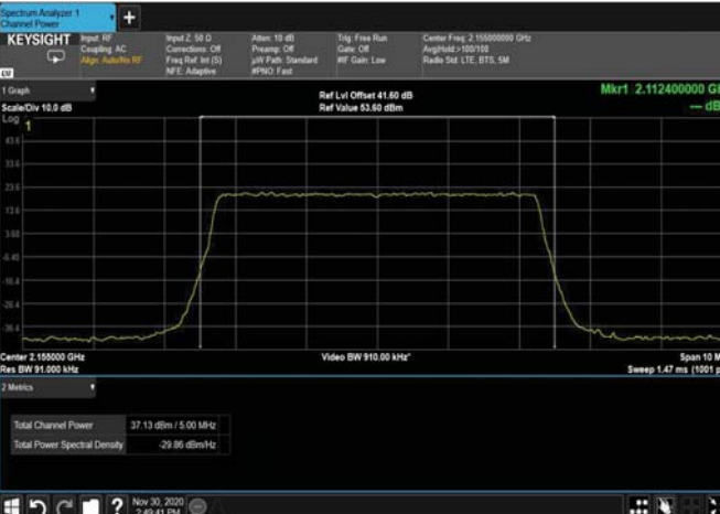
Figure 94: 64QAM 5MHz B.W; 2155MHz – 4G
