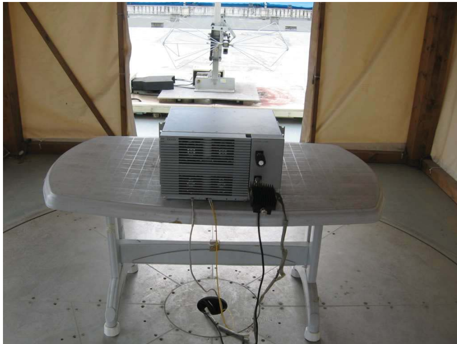
Figure 5. Radiated Emission Test 30 - 200 MHz
