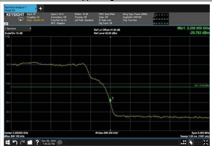
Figure 164: 16QAM 15MHz B.W.; 2192.5MHz Upper Edge – 4G
