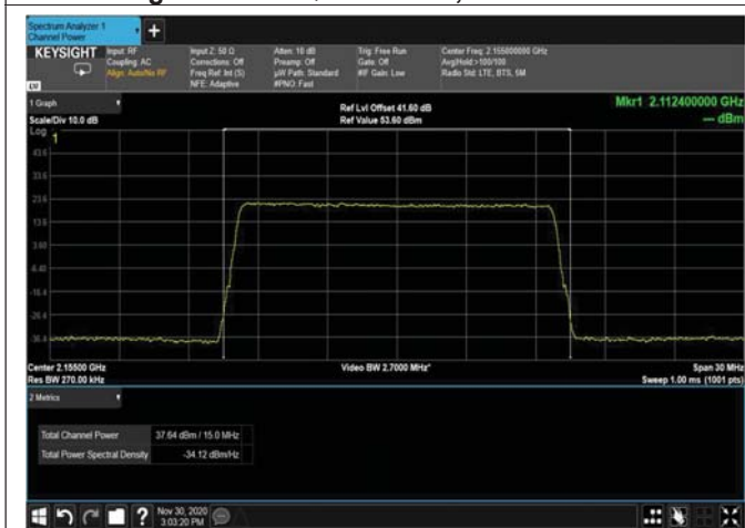
Figure 100: 64QAM 15MHz B.W; 2155MHz – 4G
