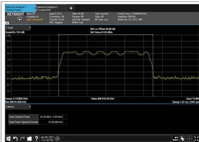
Figure 63: QPSK 5MHz B.W; 2112.5MHz, 15kHz
