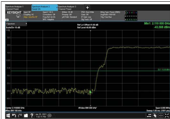
Figure 129: 64QAM 10MHz B.W.; 2115MHz, 30kHz Lower Edge
