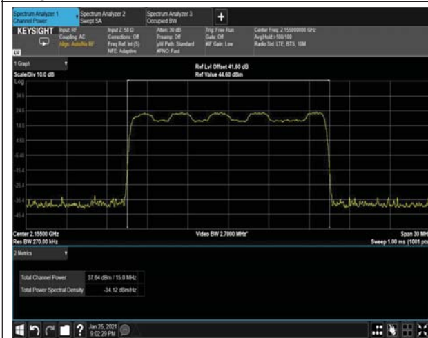
Figure 23: 16QAM 15MHz B.W; 2155.0MHz, 15kHz
