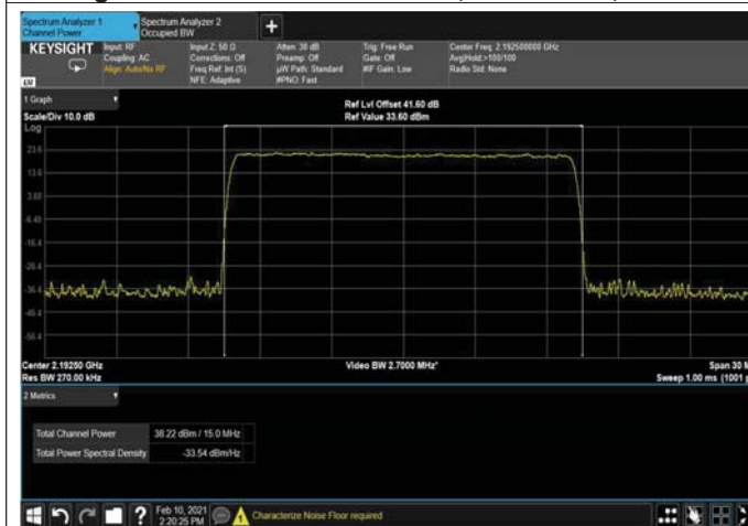
Figure 43: 64QAM 15MHz B.W; 2192.5MHz, 15kHz
