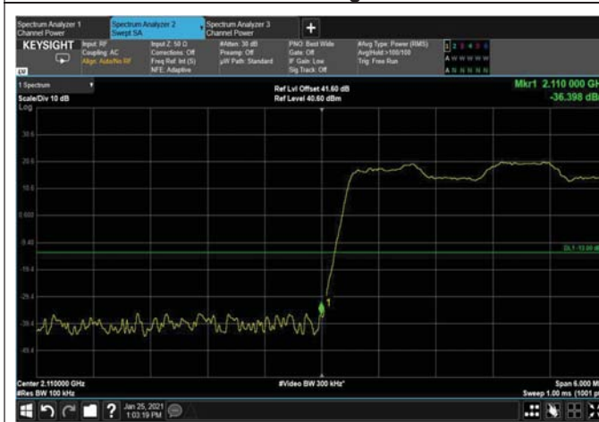
Figure 115: 16QAM 10MHz B.W.; 2115MHz, 15kHz Lower Edge
