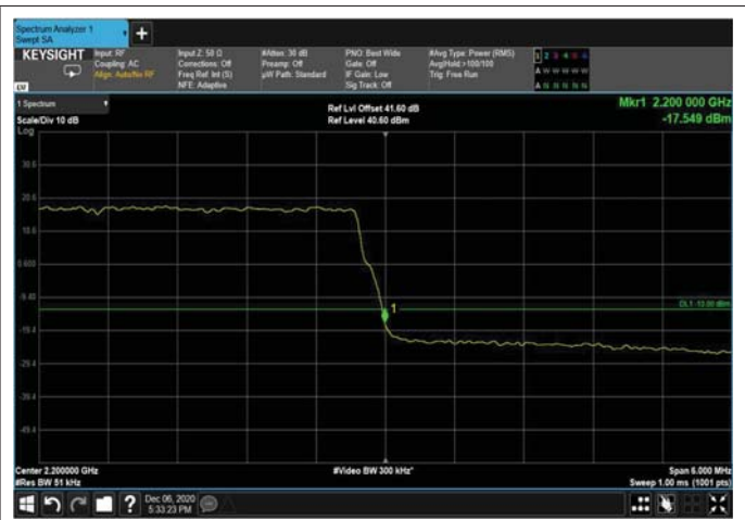
Figure 166: 64QAM 5MHz B.W.; 2197.5MHz Upper Edge – 4G
