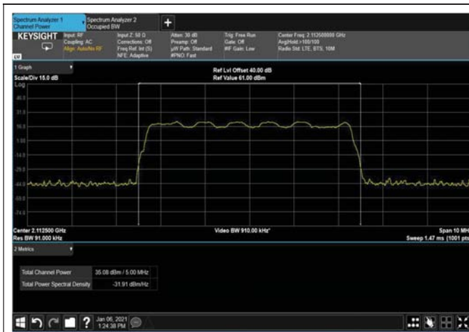
Figure 9: 16QAM 5MHz B.W; 2112.5MHz, 15kHz
