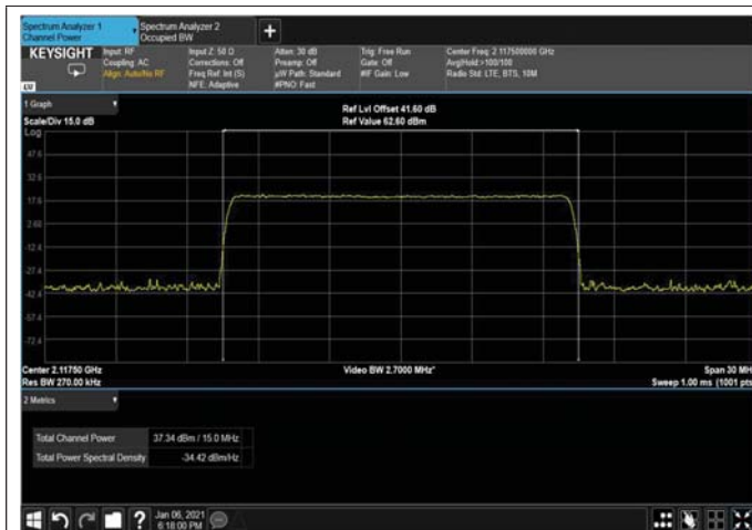
Figure 39: 64QAM 15MHz B.W; 2117.5MHz, 15kHz
