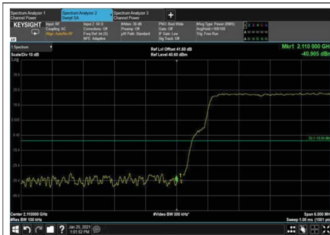
Figure 141: 256QAM 10MHz B.W.; 2115MHz, 30kHz Lower Edge
