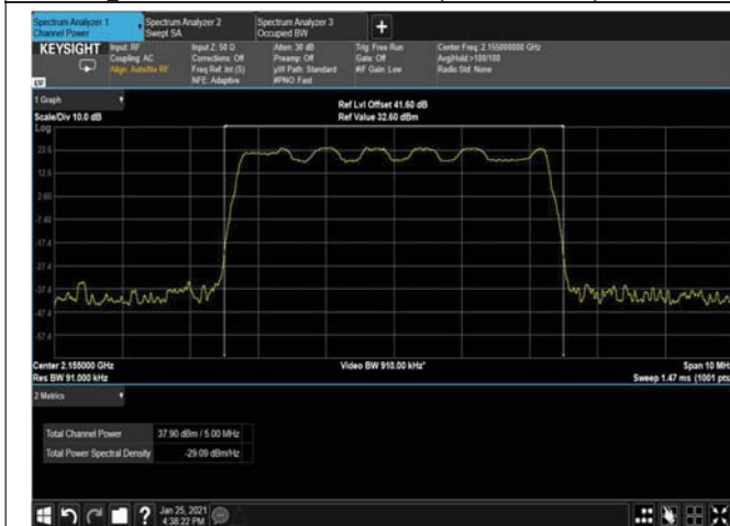
Figure 11: 16QAM 5MHz B.W; 2155.0MHz, 15kHz
