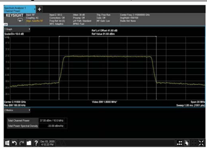
Figure 105: QPSK 10MHz B.W; 2115MHz – 4G
