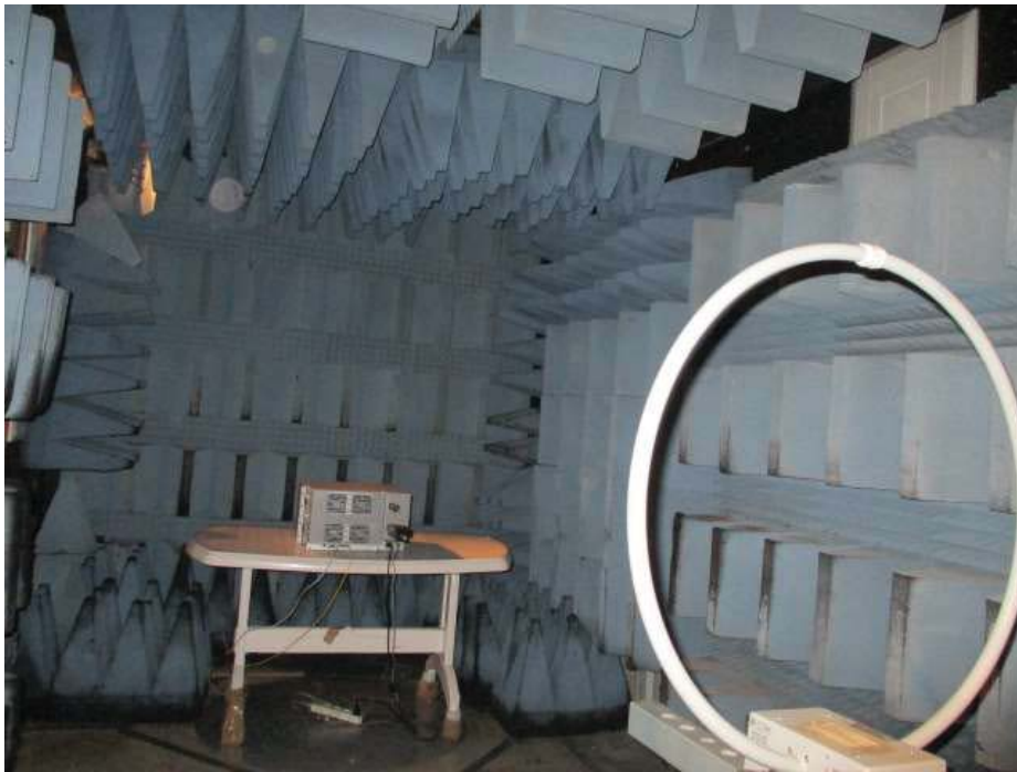
Figure 4. Radiated Emission Test 9kHz - 30MHz
