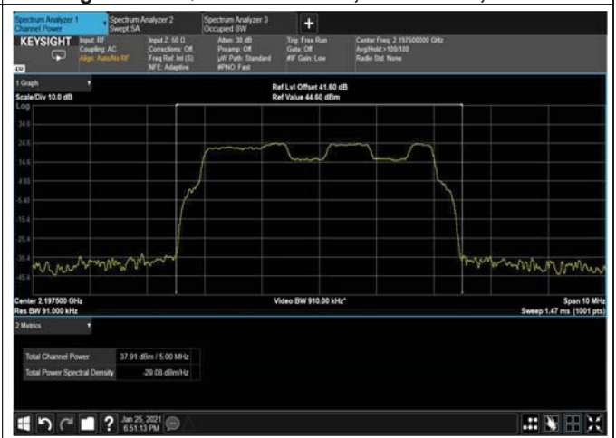
Figure 68: QPSK 5MHz B.W; 2197.5MHz, 30kHz
