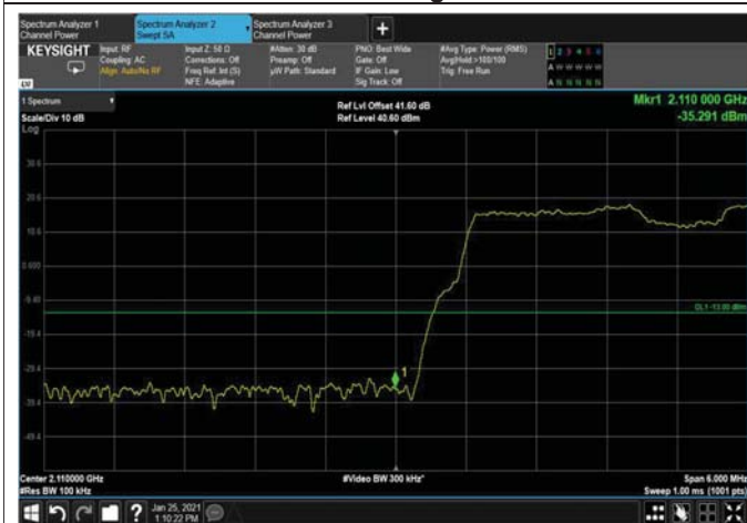
Figure 121: 16QAM 15MHz B.W.; 2117.5MHz, 30kHz Lower Edge
