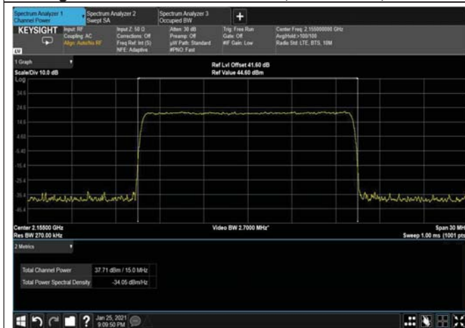
Figure 41: 64QAM 15MHz B.W; 2155.0MHz, 15kHz
