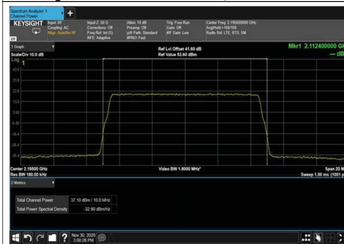
Figure 98: 64QAM 10MHz; 2195MHz – 4G
