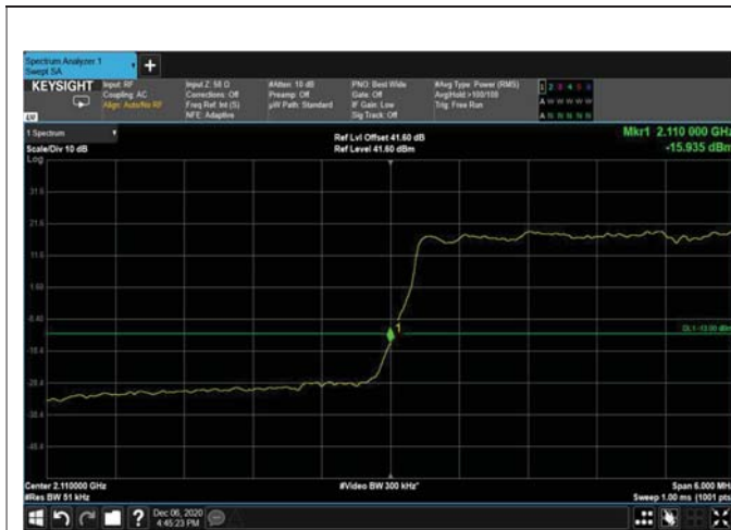
Figure 159: 16QAM 5MHz B.W.; 2112.5MHz Lower Edge – 4G
