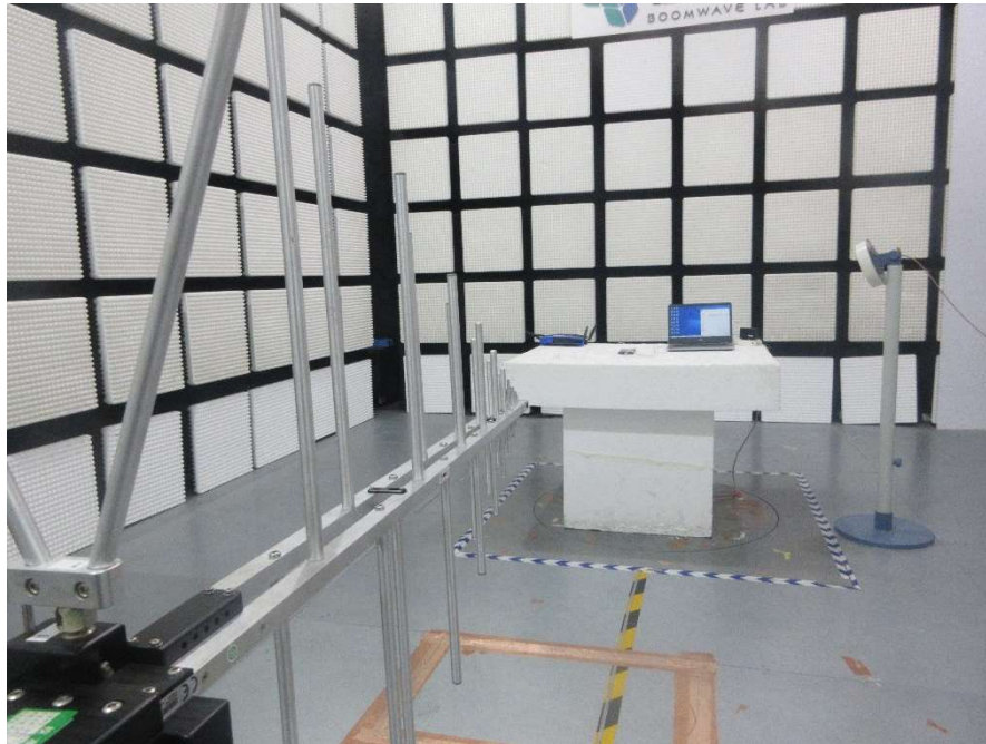
Radiated Emission 30MHz-1GHz (Front view) – Mode5
