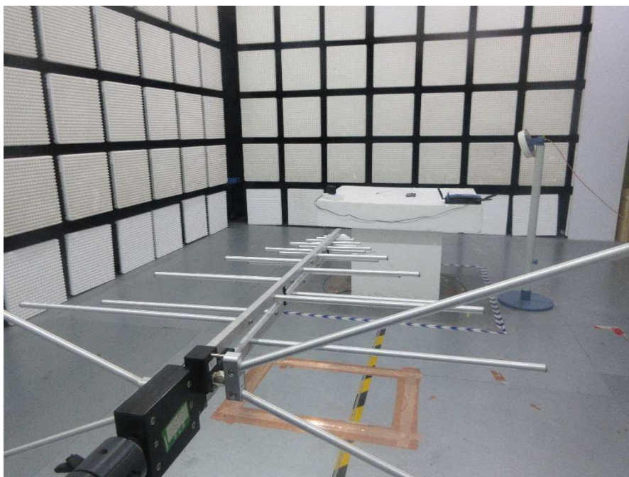
Radiated Emission 30MHz-1GHz (Rear view) – Mode2
