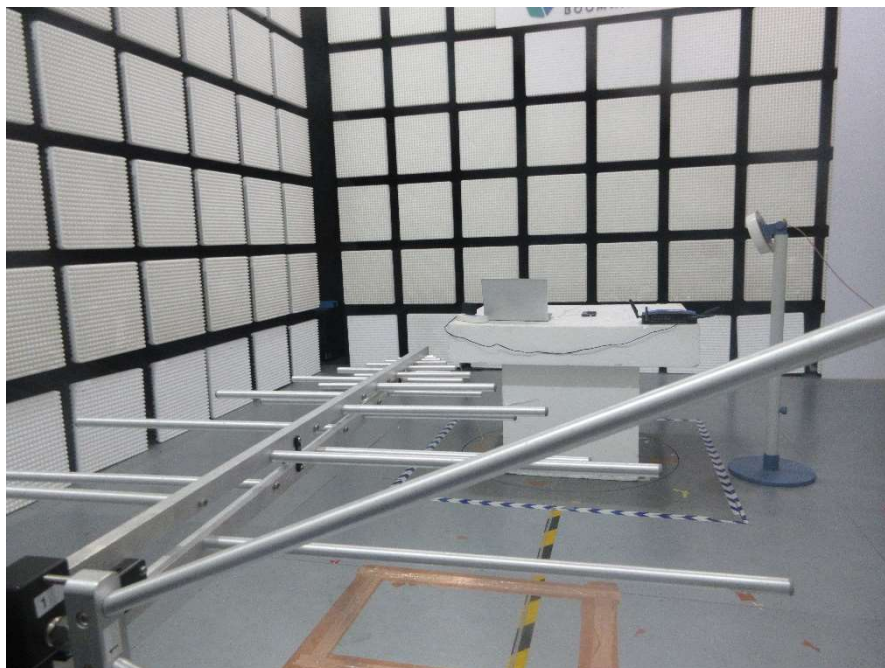
Radiated Emission 30MHz-1GHz (Rear view) – Mode5
