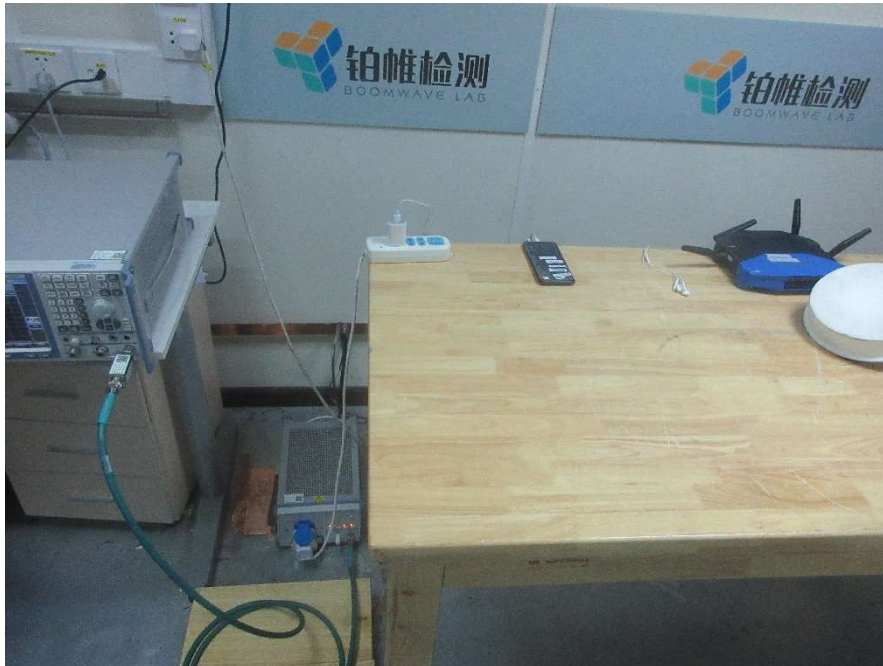
Conducted Emission 150kHz-30MHz (Front view) – Mode 2
