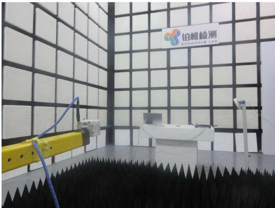
Radiated Emission 18GHz-40GHz (Rear view) – Mode 5
