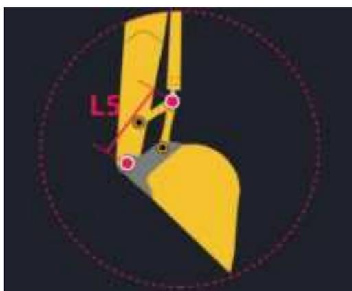
② Adjust the bucket to the center, fill in the measured L5 distance, and click check
