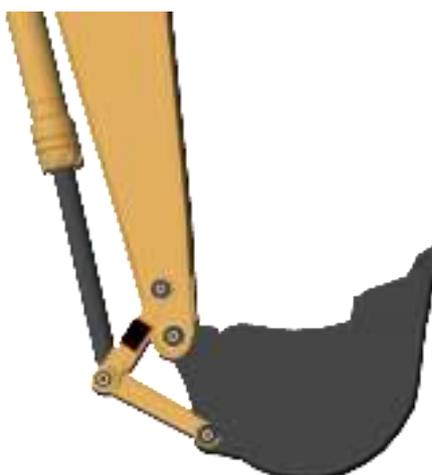
Attach the sensor to the bracket using the screws, the sensor arrow to the bucket and the indicator to the cab
