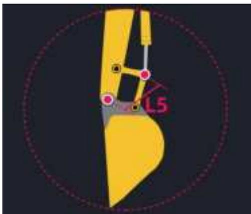
③ Adjust the bucket to the adduction limit, fill in the measured L5 distance, and click check
