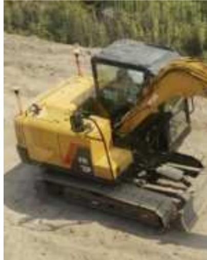
**Note: for more than 20 tons, the distance between the two antennas should be kept above 1.5M**
