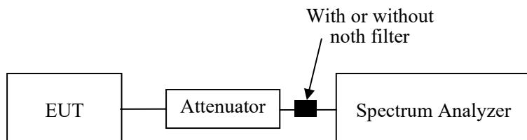
Note: the path loss(cable loss and attenuator) has included into the plot.
