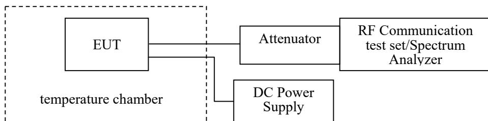
Frequency Stability vs. Temperature: The equipment under test was connected to an external DC power supply and the RF output was connected to a Frequency Counter via feed-through attenuators. The EUT was placed inside the temperature chamber. The DC leads and RF output cable exited the chamber through an opening made for the purpose.
