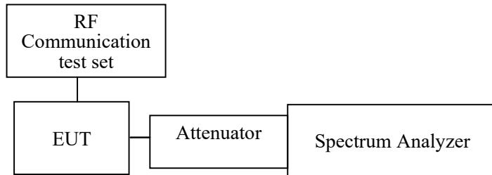
Note: The path loss from EUT to Spectrum Analyer has included in the result.
