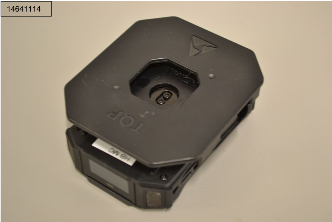
Photograph 7: Back View of the DUT with Wing Clip Mount
