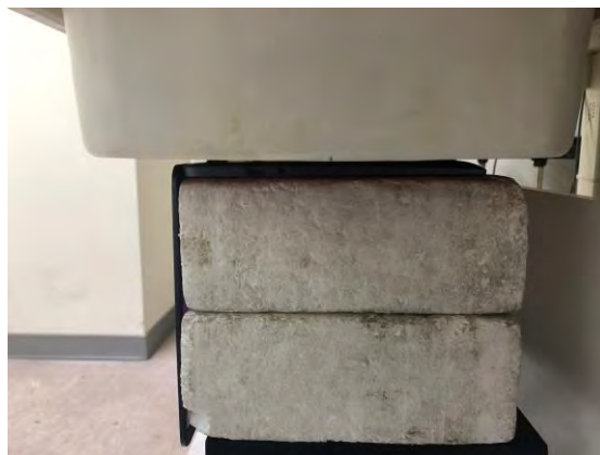
Fig.3 EUT Bottom side to flat phantom
