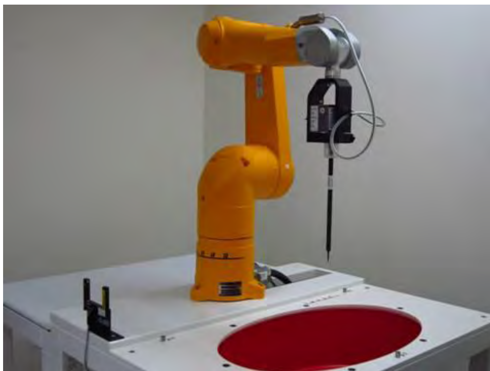
Fig.1 Photograph of the SAR measurement system
