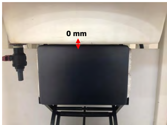
Fig.3 EUT Bottom side to flat phantom
