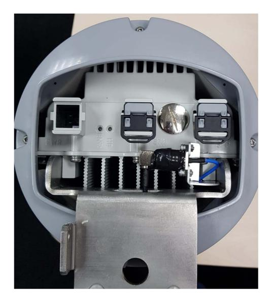
Photograph No.5 "AirSpeed1050 2.6 GHz (B41)" base station removed from case, top view
