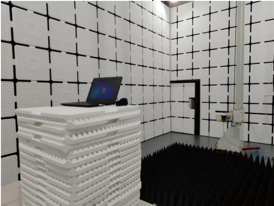
Radiated Emission Test Setup Photo - Above 1GHz
