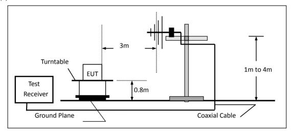
(c) For radiated emissions above 1000MHz
