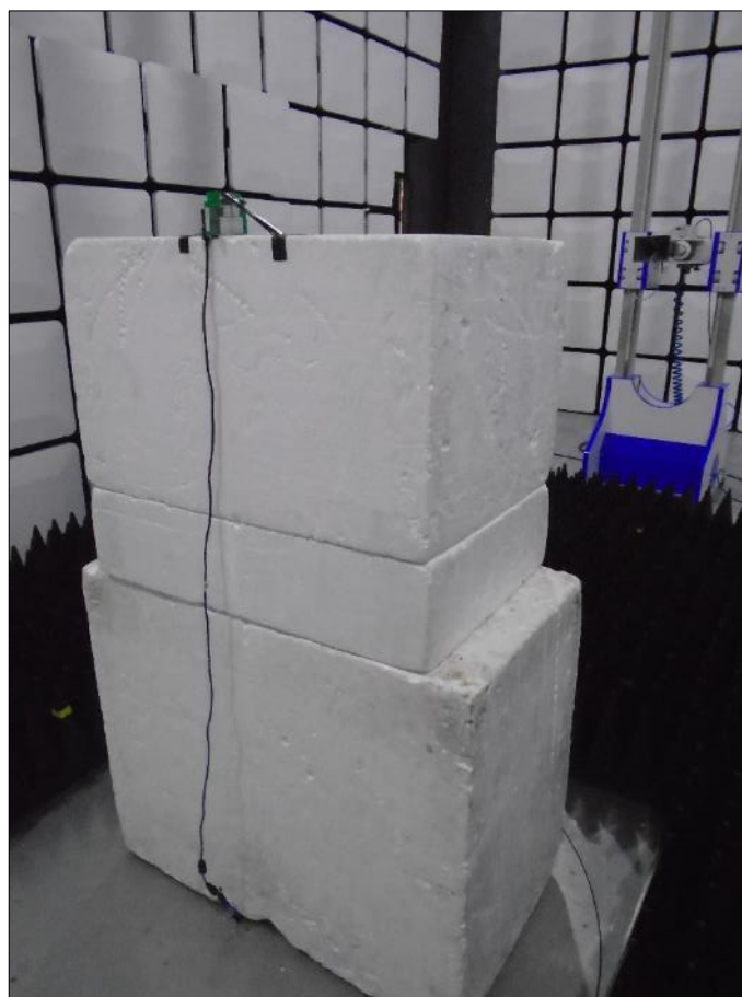
Figure 255 - Test Setup - 1 GHz to 10 GHz - Z Orientation
