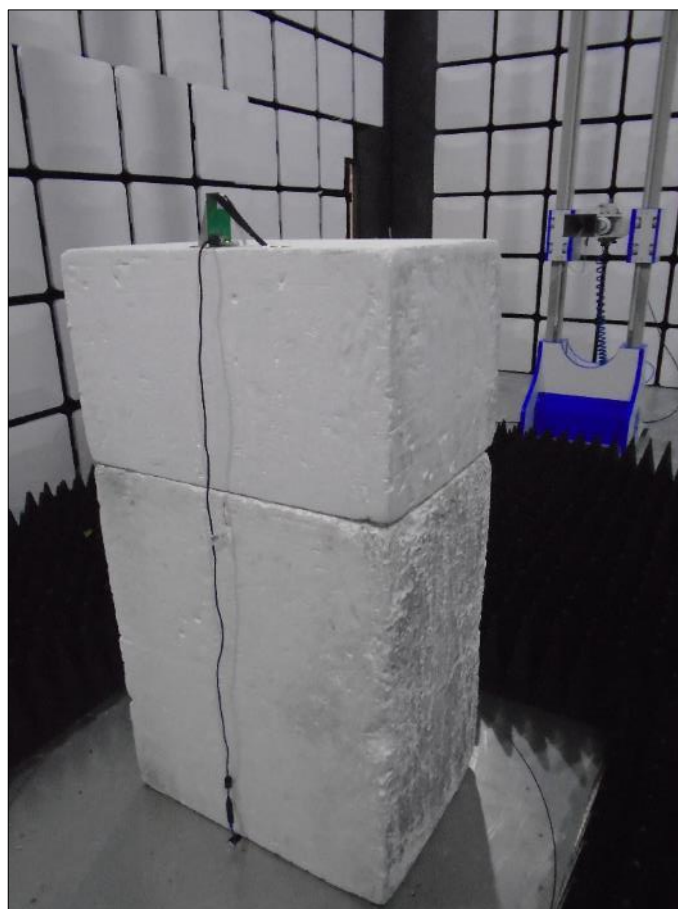
Figure 254 - Test Setup - 1 GHz to 10 GHz - Y Orientation
