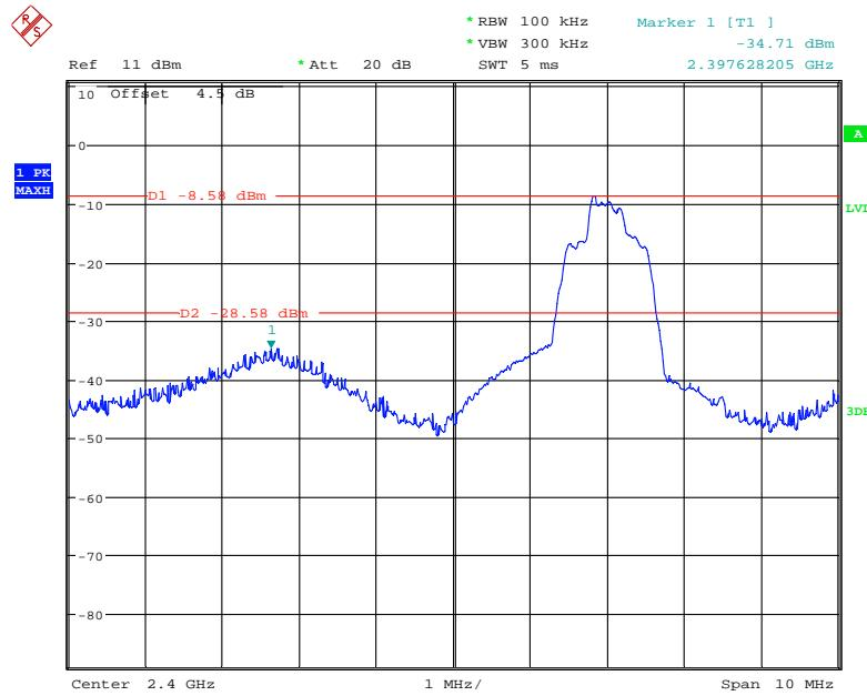
**EDR ( $\pi/4$ -DQPSK): Band Edge-Right Side**
