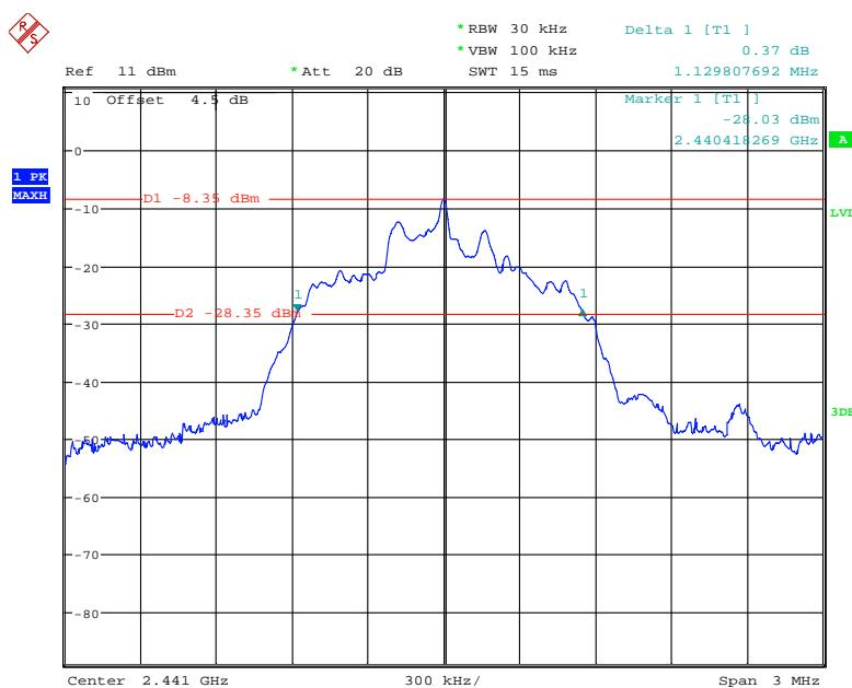
**EDR (8DPSK): High Channel**
