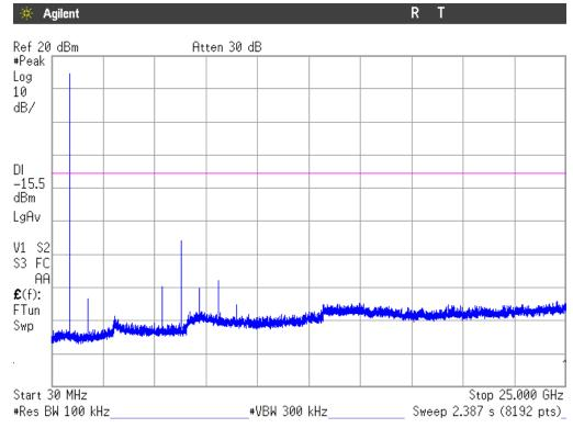
Note: The peak shown in the plot above the limit is the carrier frequency.
