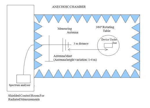
Radiated measurements setup f > 1 GHz
